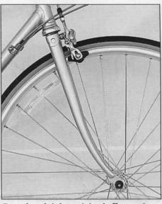
Even though it has minimal effect on how the bike rides, we insist on a nice-looking bend in the fork. Notice the low radius, and how the blade continues to bend all the way to the dropout. Few modern forks look this good. Way less than half.
