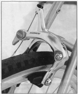
The Romulus has Shimano standard reach brakes, and a properly placed brake bridge, to maximize tire and fender clearance. Also note the rack mounts inside the seat stays.
