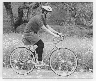
to let you simultaneously have the saddle at the proper height, get the bar at least as high as the saddle, and still be able to straddle the bike comfortably. Most bikes don't allow this. They are not as well designed. Don't scoff at Mark's shoes. He's still faster at 44 than Grant was at 28 (and I was fast then).
