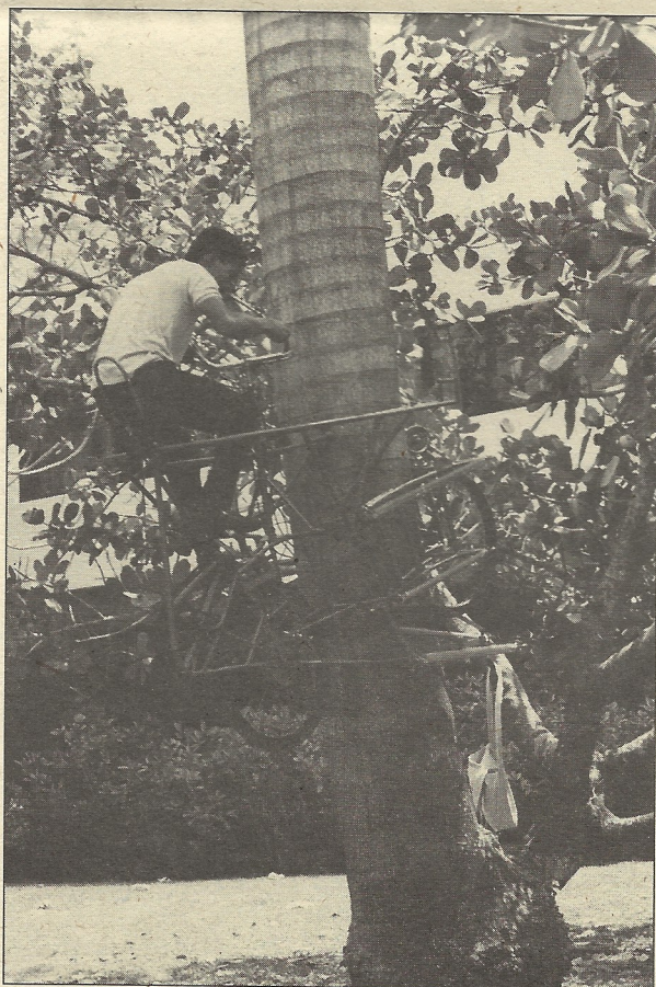
The Cyclopalma: This man-powered tree climber (for picking palm-nuts) gets a flat tire every time up. Other than that, it works great.
