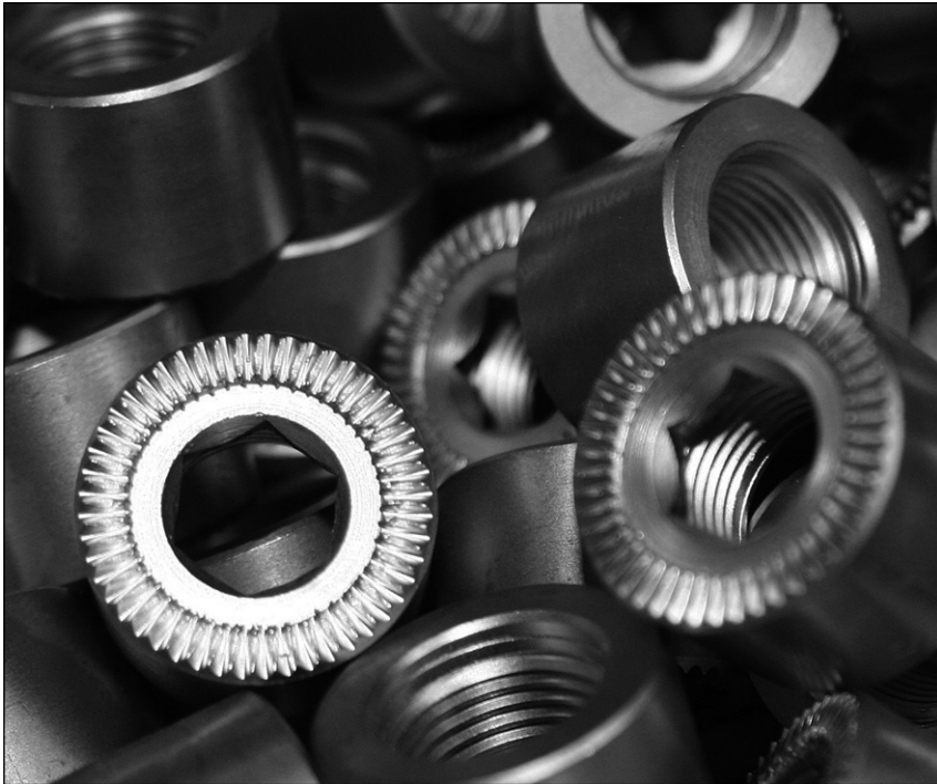
Finished endcaps. These are the cylinders just outside the hub flanges. They thread onto the hub axles (see the hex holes) and butt up against the dropout faces.
