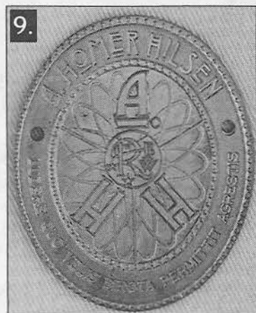
Here's a badge after the first squeeze in the hydraulic press shown to the left there. A closer inspection will reveal some of the flaws from the first squeeze where the borders aren't fully even.
