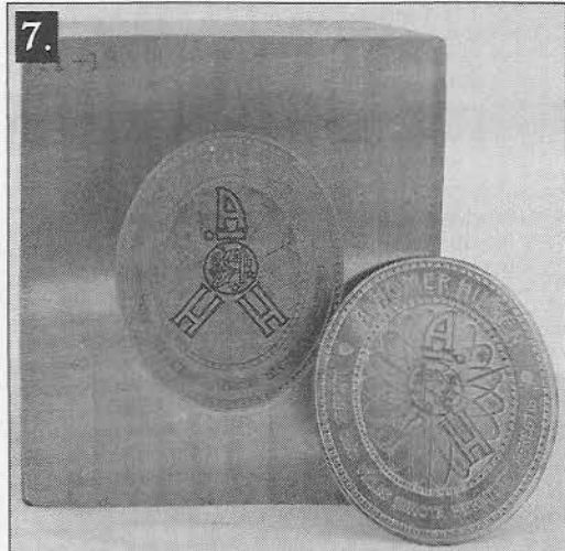
Here's a badge after the first squeeze in the hydraulic press shown to the left there. A closer inspection will reveal some of the flaws from the first squeeze where the borders aren't fully even.
