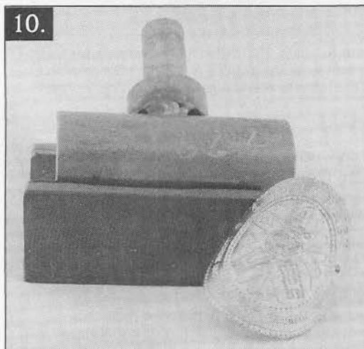
Finally, we make a "dapping" tool, which forms the badge to fit the bike's head tube. The lower part of the tool is wood, radiused to fit snug against the head tube.
