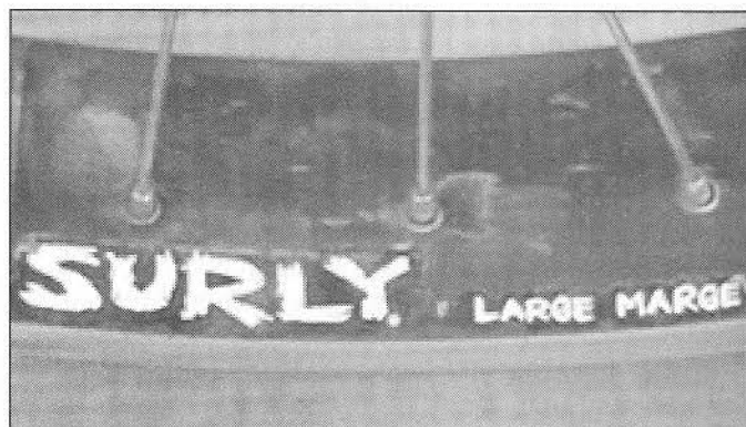
The Large Marge rim has offset spoke holes and is wide enough to hold the Endomorph, even at low pressure, without rolling. It's one of many ultra-fat specific parts made for the Pugsley, and it must be the most unwreckable rim ever made for a bicycle.
