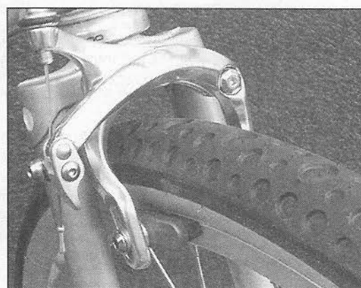
At about 40.5mm, this Fatty Rumpkin is currently the fattest 650B tire suitable for the Silver brake. By adjusting the brake with the Q/R up, you can easily open up the brake pads to clear this tire. Using brake levers with integral quick-release buttons is another way to go. Not a bad way, actually.
