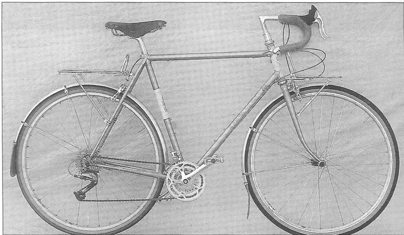
A be-fendered A. Homer Hilsen ready for bags, baskets, whatever you got. Stuffed with function and good design, it's a beaut to look at, and it gallops over everything it sees. The final one will have mid-stay braze-ons for the rear rack, double-tapered seat stays, and a non-paper head badge.
