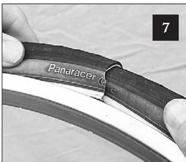
7 Fitting it again. Just checking. Lining it up (the overlap).
