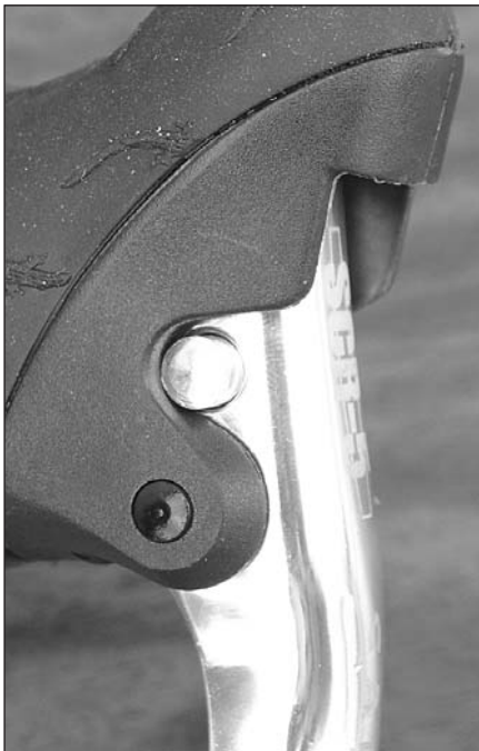
QUICK-RELEASE ON. With the button pushed over to the right, the lever retracts more, feeding more cable to the caliper. This is a really good feature. It's not a "must have" by any means, but it's not a sissy feature, either. It's right in between.
