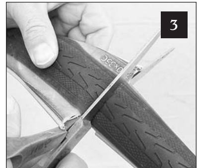
3 After cutting both beads, cutting the tread with scissors.
