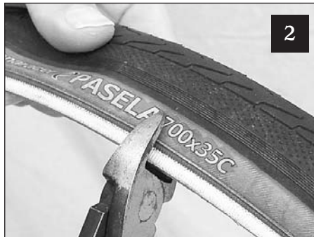
2 Cutting the wire bead with dykes.
