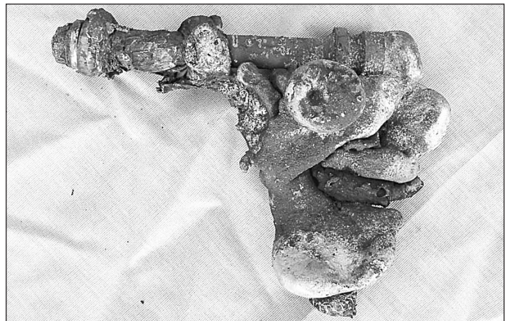
Campy Chorus rear hub. If it couldn't take the heat, it should've stayed out of the bike locker.
