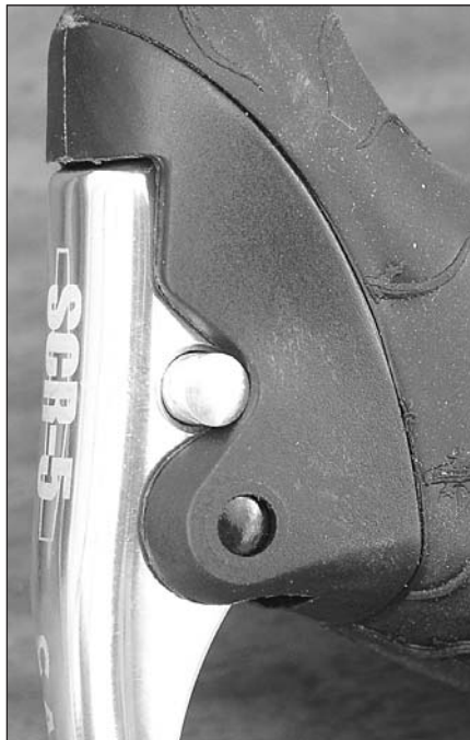
QUICK-RELEASE OFF. The normal position, for riding. The q/r button is pushed to the right, and this side of the lever body isn't as deep as the left side, so the protruding button gets caught sooner.
