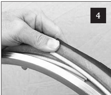
4 Fitting the whole cut tire on the 603 rim, showing the overlap.
