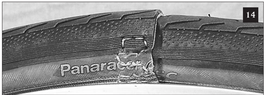
The stitched-up tire from the outside, almost too pretty to look at. Makes you want to take off on a long, treacherous, high-speed descent, doesn't it? Me three. Panaracer must be proud.
