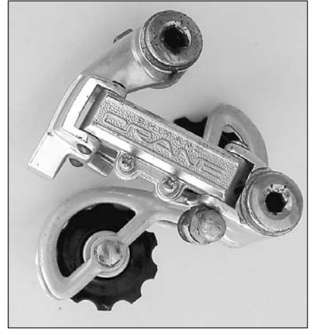
Shimano's first "pro" derailleur, the Crane, part of the first Dura-Ace group in 1973. There was never a "Crane" anything else, just this. It shifted better than Campy's best, but didn't index.
