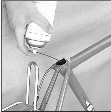
Seat tube and top tube. Remove seat post and you can get at both the top tube (you'll see the hole) and the seat tube. But not simultaneously!
