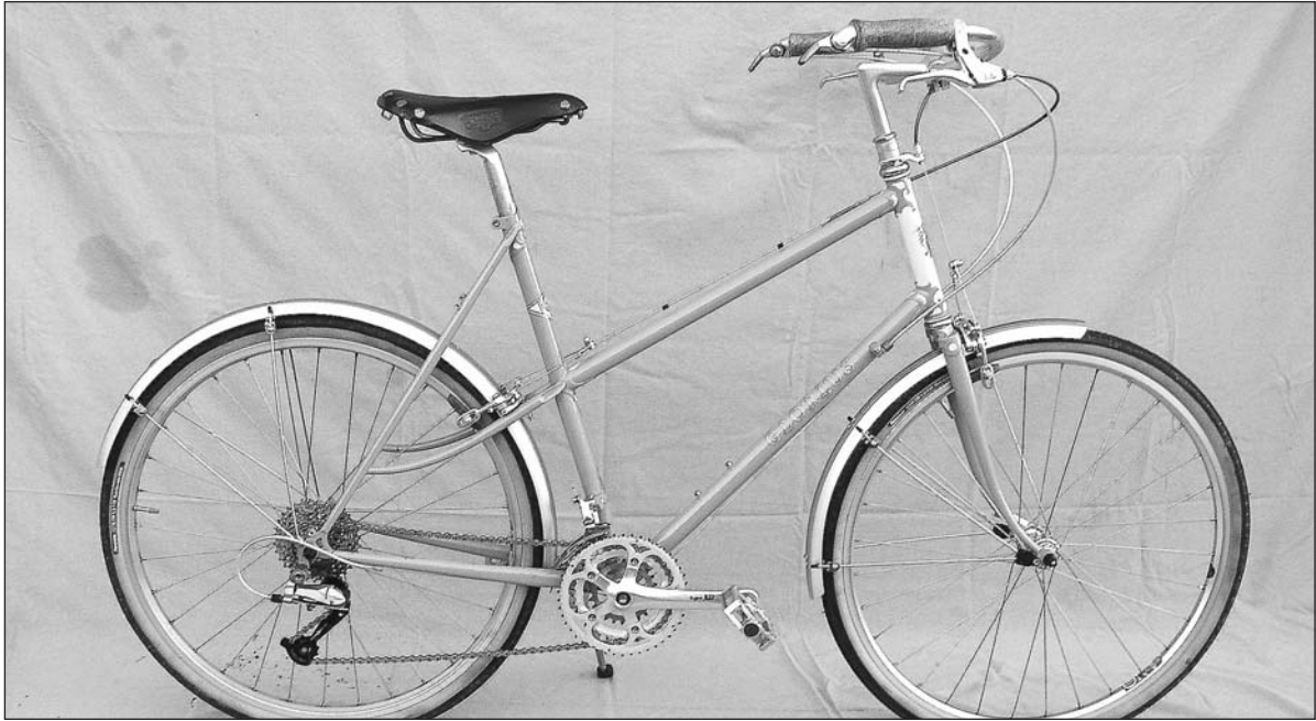
A 56cm Glorius set up for comfortable, upright riding. That's an 11cm stem. You can set one up with drops if you like, just use a shorter stem. Ideally, this bike would have a wider saddle, but we didn't have any at photo-time.
