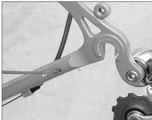
Chain stays. Find the vent holes near the dropouts and spray away. It is easier, but not necessary, to take the wheel out. Same as fork blade.
