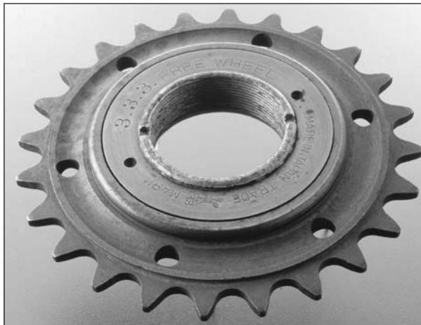
One of the early freewheels. Shimano still makes single-speed freewheels.
