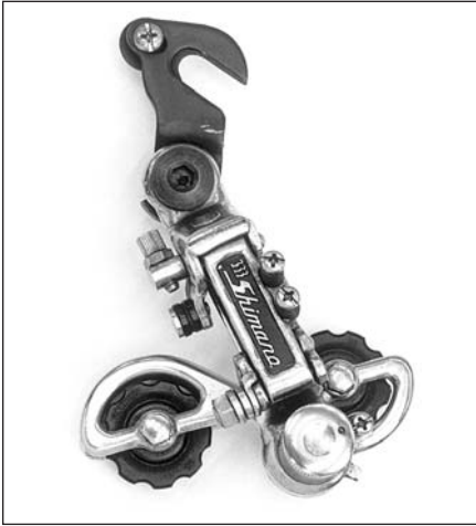
Shimano's first rear derailleur, the 3.3.3. Introduced 1965.
