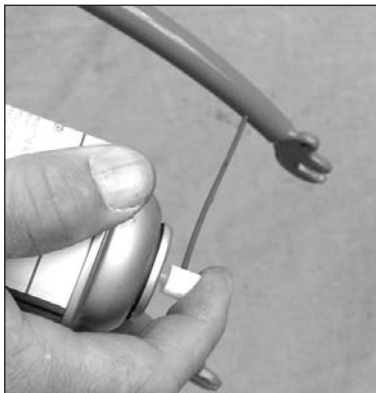
Fork blades. Most real forks have brazing vent holes somewhere on them. Usually two per blade, one high and one low. Look hard!
