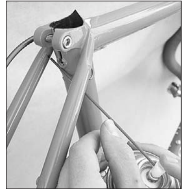
Seat stays. Often there are brazing vent holes. Sometimes builders fill them in, but we don't. On this bike, see also the rack mounts.
