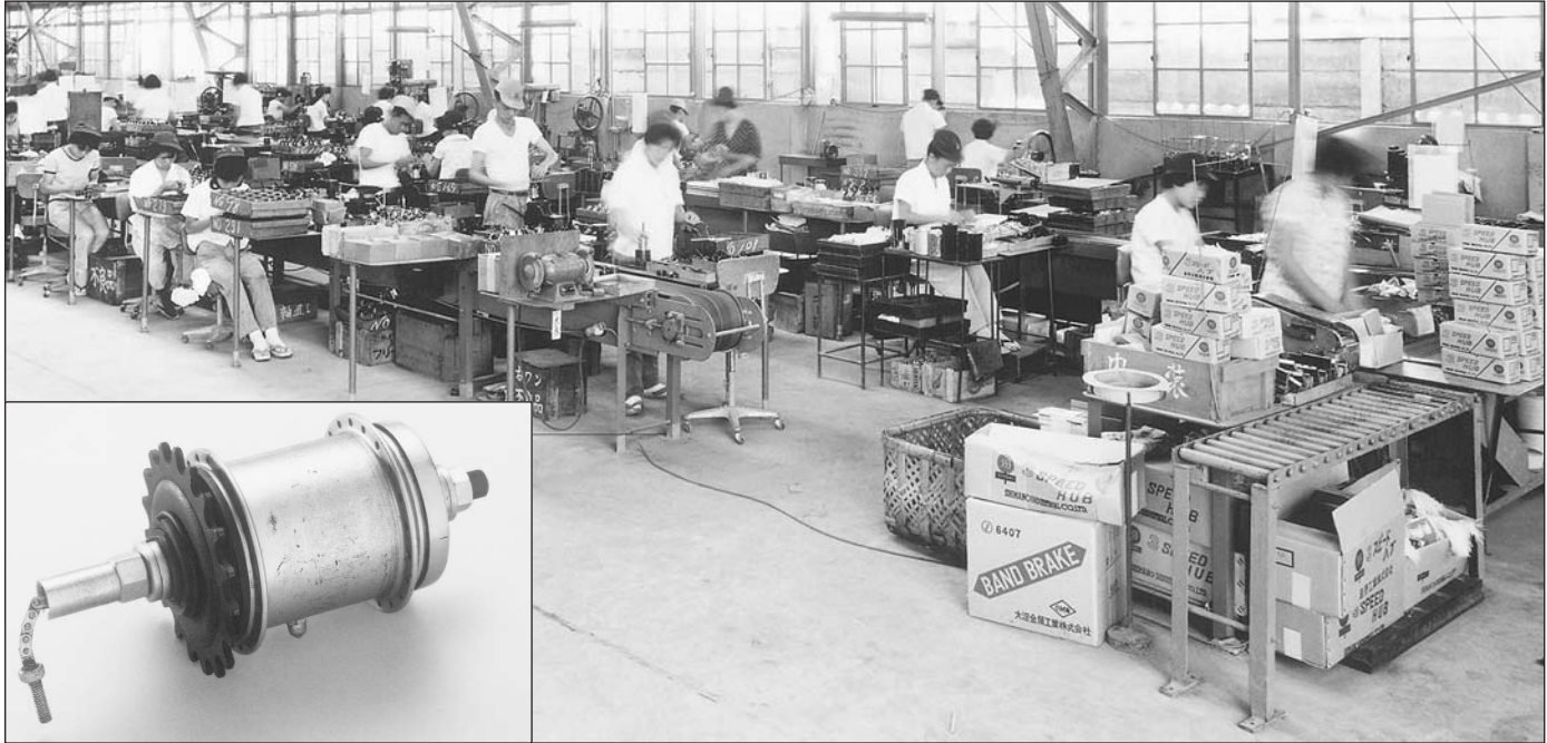
Assembling 3-speed hubs and, presumably, band brakes in the early '60s. Shimano still makes 3-speed hubs and band brakes.
