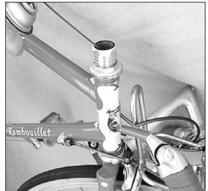
Head tube. The least likely tube to thank you for spraying, but you might as well. Remove the stem first. Don't let it drip onto the tire.
