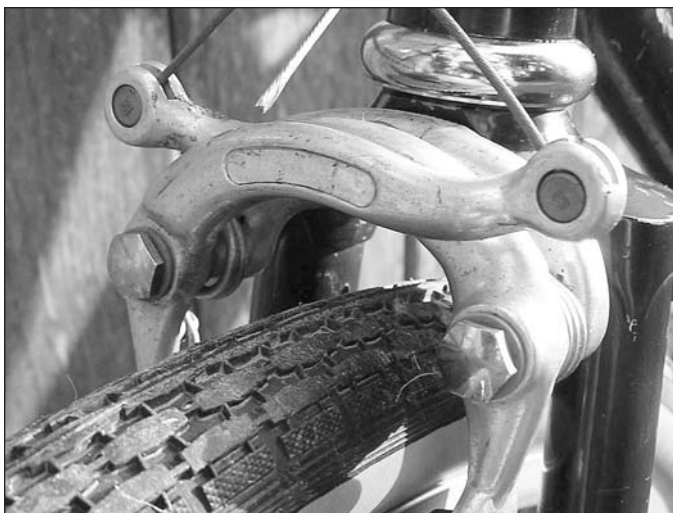
The front brake shoes are at the bottom of the slot, because the reach on this brake is shorter than it is on the rear. It barely reaches the rim, but "barely" is still a bullseye. There's easily room for a fender there, even with the 650B x 38 tire. There'd be even more room with a Michelin Megamium, 650B x 32. With 700c wheels, the bike fits only a skinny tire, and no fender.
