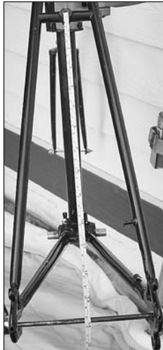
MEASURING. In the photo above, although you can't see it, the tape is in the center of the brake hole in the fork crown. You can see that the hole-to-axle distance is 355mm (see where the skewer sits in the dropout). Right: Full view of the equivalent measurement on the rear part of the bike.
