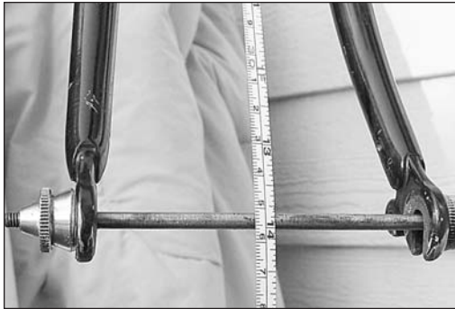
MEASURING. In the photo above, although you can't see it, the tape is in the center of the brake hole in the fork crown. You can see that the hole-to-axle distance is 355mm (see where the skewer sits in the dropout). Right: Full view of the equivalent measurement on the rear part of the bike.
