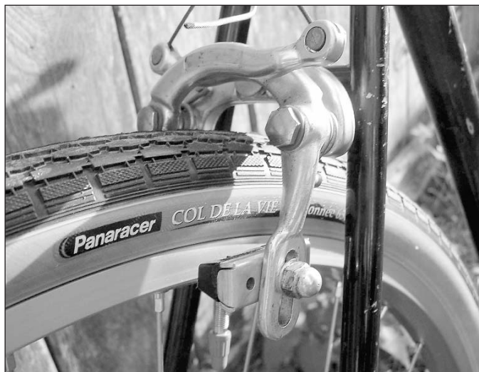
For the rear brake, I used a longer Dia-Compe Mod. 750 model, to account for the rim movement when using the full length of the adjustability of the horizontal rear dropout. This would make a better brake for the front, too—but I don't mind the slight mismatch. Also plenty of fender clearance—
