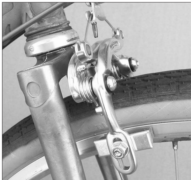
This prototype Saluki (unpainted and well-ridden) has a cantilever rear and a centerpull front. We also have a spare fork for it, with a cantilever on it. We won't mix brakes on frames; we're just testing. We'll use a longer straddle wire on the centerpull.
