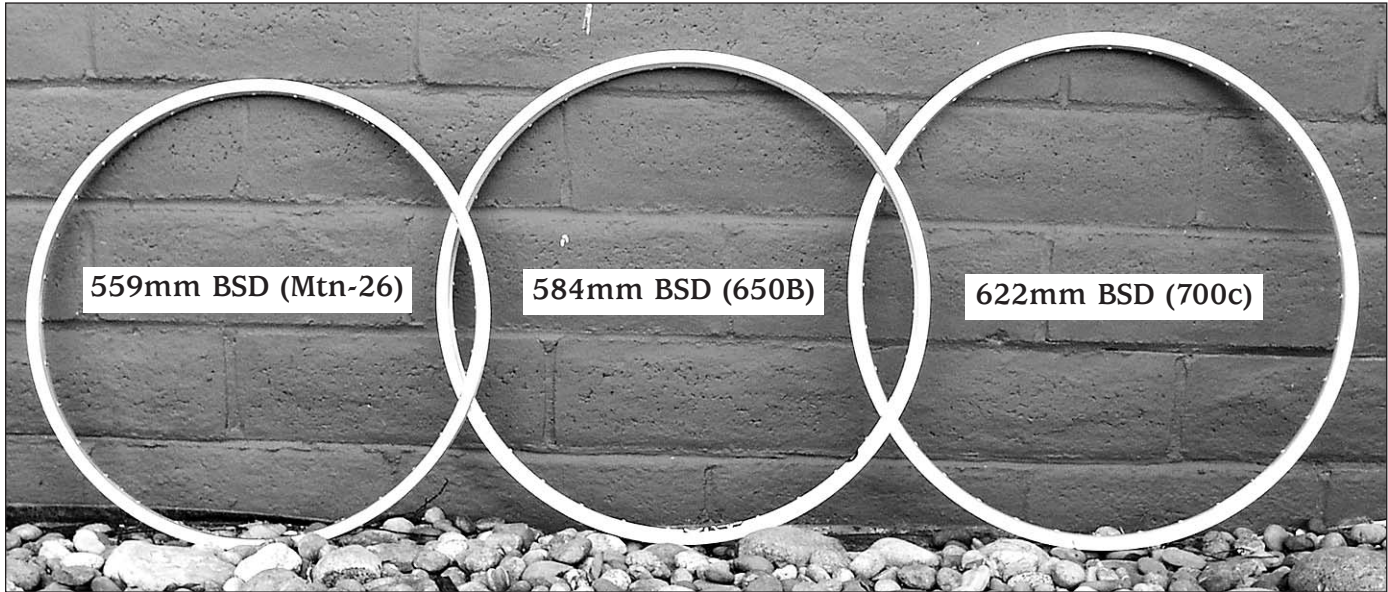
The three wheel sizes discussed here are shown above. BSD stands for bead-seat-diameter, which is how rims and tires are specified by makers. It would avoid a lot of confusion and duplicate language if all riders were familiar with these numbers.
