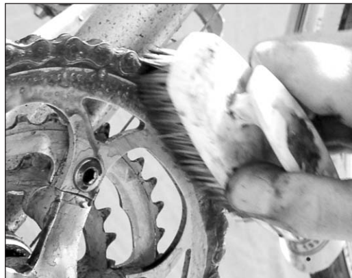
After the cogs and chain and pulleys are pretty clean, go over the chain again, paying more attention to the side plates. Do it like this, and you'll also clean the chainring. Go at the others, too.
