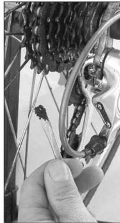
STEP ONE. Use the screwdriver to clean the major gunk off the pulleys. Easiest with bike in a stand, pedaling to rotate the pulleys.
