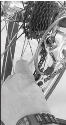
STEP ONE. Use the screwdriver to clean the major gunk off the pulleys. Easiest with bike in a stand, pedaling to rotate the pulleys.
