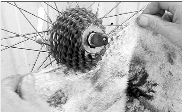
When the cluster is fairly clean on the outside, it still has built-up gunk deep between the cogs. Remove the wheel and using a raggy towel (also not shown in the first photo), floss deeply in each groove. This is the most satisfying part of the process, and it is not actually that satisfying.
