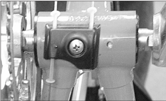
Soft-focus picture of the underside of the BB shell. The shell was stamped, with no effort made to spiff it up. Internally, we called this a "chop-chop" shell, because the chainstay sockets looked like they'd just been chopped off straight and brazed up. This was norm for bikes of this quality. It's not a terrible thing, just reality. Notice the well thought-out cable guide.
