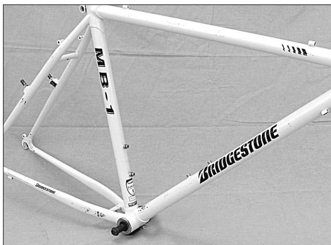
The MB-1 was a good frame between 1986 and 1994. The early ones (through '87) were slacker than the later ones, but they all rode well. This frame will be rebuilt with Albatross bars.
