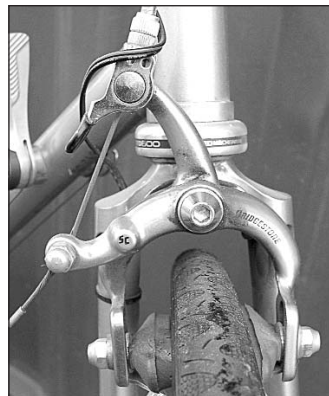
The Bridgestone SC brake. This unique brake was made by Dia-Compe, but was a Bridgestone design. The SC stands for self-centering, and it worked great. No matter where the wheel was, when you applied the brake, the brakes would automatically center themselves around the rim upon release. It was really smart, and still is, and if this brake were reintroduced in a spiffed-up version by Shimano or Campy, holy cow, it would set a new standard. But Bstone had this middle-of-the-road version. It worked well, but wasn't distributed as an aftermarket brake, an certainly couldn't compete against the top sidepulls of the day. A pair cost about $25 to $35. Nobody was going to take off Campy to put on this. It is a super design despite its lack of commercial success. Imagine it with a micro-adjust q/r, fine finish, and a Shimano label. It would set a new standard, I think.
