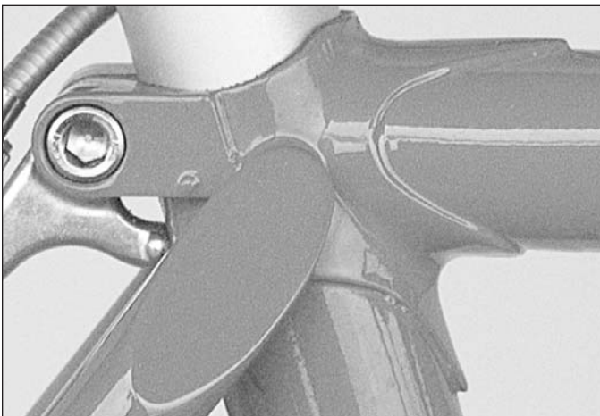
The XO-1 seat lug, like all Bstone seat lugs, is stamped. In this case, the binder portion is brazed on separately. See the seam? We had a lot of customers say "it looks like a crack," but it wasn't. This is perfectly acceptable on a bike of this overall quality.
