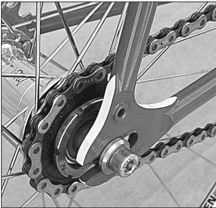
Track dropout with creamed points. The threaded eyelet makes fenders easy.
