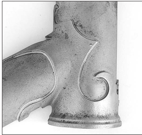
Lugged. The tubes aren't heated enough to melt. Reinforced with extra metal. Won this test, but not the only good way to make frames. Not the way of the future.
