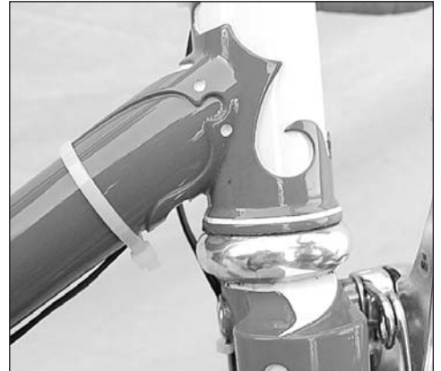
The head lugs have the same custom cutting as the seat lug. The crown wave is painted cream.
