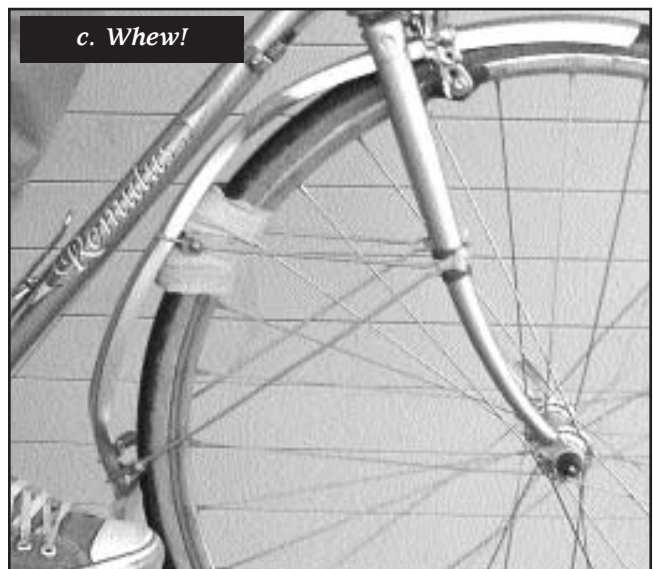
THE BRITISH WAY: Fenders mounted to the fork's midpoint without using a quick-release. Usually this is done with a braze-on, and on our customs we put a braze-on there if you request it. But as long-time readers know, we're enamored with zip-ties, and here's yet another reason why. As you can see, the jamming forces the fender away from the tire, just the opposite of the photo to the left. The fender does NOT accordion, and this is not nearly as likely to send you over the bike. This is not officially called "the British way," but most of the bikes I've seen with high-mounted fender have been British, so there you go.
