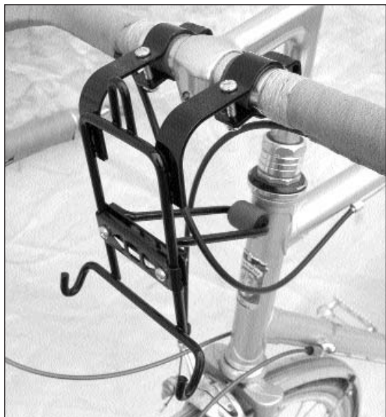
Here's the genius-ish part, the mounting bracket. We wrapped the stabilizer with bar tape so as not to wreck the head tube. Comes with clear instructions.
