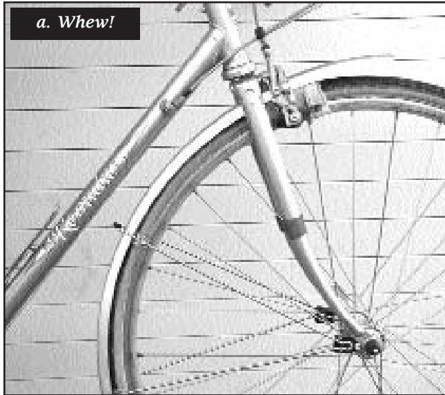
PROPER, NORMAL, SAFE. Look at the lower attachment point. These fenders, SKS brand, have a quick-release. The stays have pulled out of the plastic retainers, and the fender is loose, but nothing jams up, buckles the fork, and pitches you on your head.
