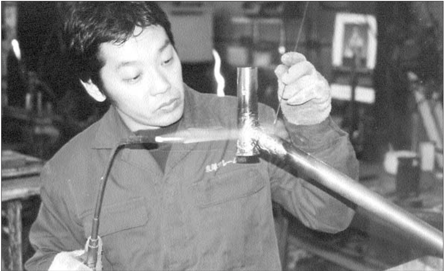
Head designer, builder, and son-of-founder Tetsuya Ishigaki brazes a Rambouillet. Sometimes he wears dark glasses.
