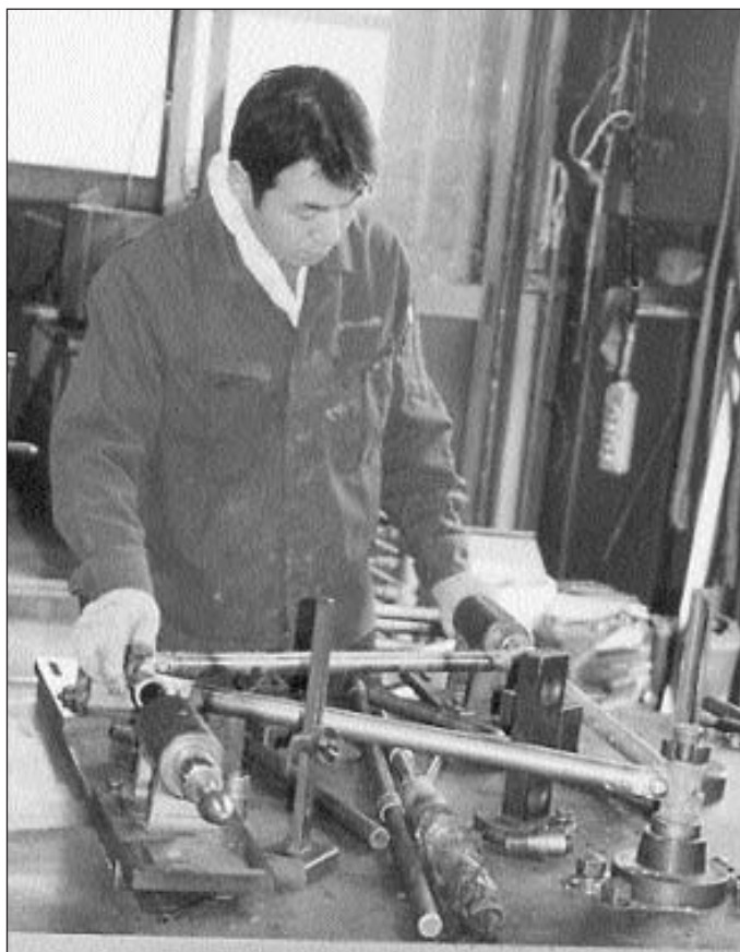
Checking a frame for alignment. Toyo frames are always straight.
