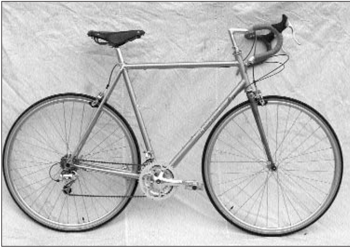
Straight forks, eek! Not a good look in my book, and with no offset (rake), it resulted in a world record 105mm of trail. The bars are tilted too much here. I didn't ride it thataway...
