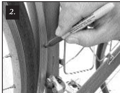
2. Using a Sharpie, mark a good spot for a hole for the zip tie, which will pull the fender off the tire. On race bikes with short chainstays, you gotta do this. Make two marks, one on each side.
