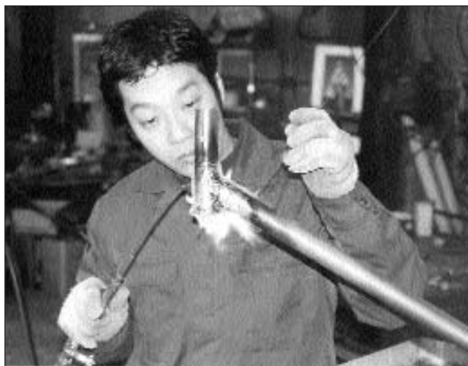
Tetsuya Ishigaki brazing the first joint on a frame—the lower head tube to the down tube. He feels that this is the most critical joint for maintaining the specified geometry.
