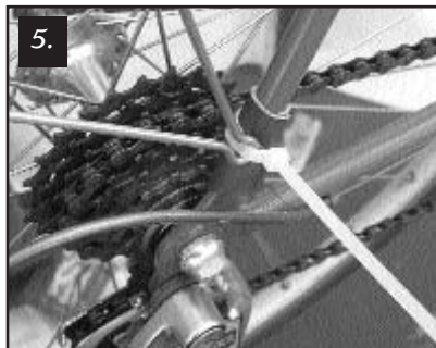
5. Zip-tie the fender stay to the seat stay, if there are no eyelets. This one here is padded with scrap of Naugahyde scrap. You'll find that Zip-Ties + Naugahyde were made for one another!
