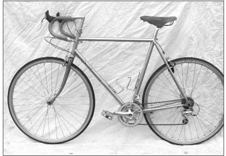
Just to keep things lively, we built up this bike left-side drive, right down to the decals. 65mm of rake, only 37mm of trail. I quite like the look of lots of rake.
