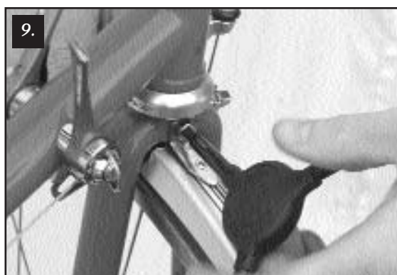
9. Tighten the 5mm nut so it holds the fender on.
