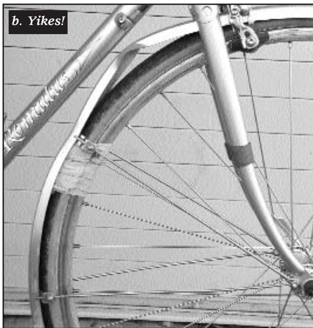
THE DEADLY WAY: Fenders mounted to the lower fork without using a quick-release. An obstacle caught jams between the tire and fender, buckling the fender and pulling it down onto the tire, locking the wheel. At high speed, the fender would continue to fold, like an accordion, and you'd be pitched forward. Aluminum fenders are probably less likely to fold than are plastic ones, but the physics don't care what the fender's made of, and if the object is big enough and you're going fast enough...
