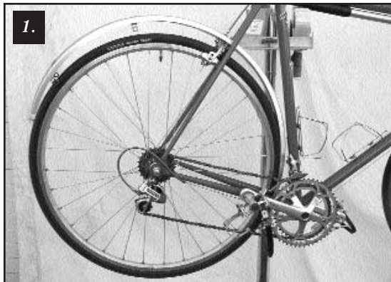
1. Put the rear fender in place, and over the brake.
