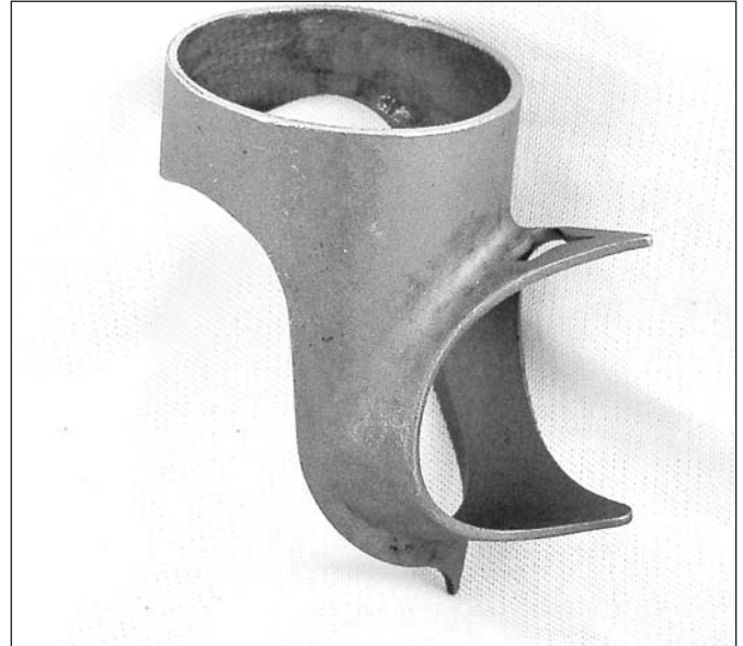
Richard's new top head lug matches his other ones, and has a smart extension cast into it.
