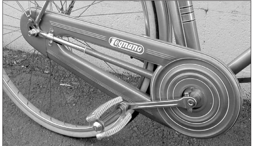
Above: The fully enclosed chain case prevents amateur marks on your calf, and keeps the elements from attacking the chain. Some bikes back then had oil baths in the chaincase, so the chain stayed lubricated forever and never wore out. I don't know whether that was the case with this Mod. 44, but let's just pretend: The chain ran through an oil bath at the bottom of the chain case, so you never needed to lube it!
