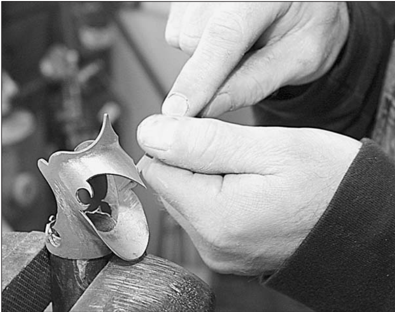
Filing an early Rivendell lug. We supplied Richard with lugs for some of his bikes. Only fair, since he designed them.
