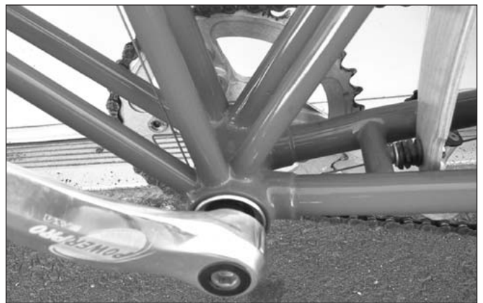
The bb area showing how the heck all the tubes come together.
