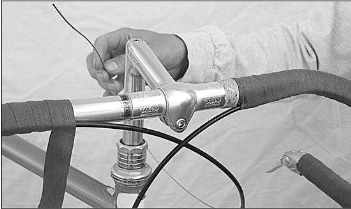
Unhookup the brake cable. Pull it back through so it's at least out of the portion of cable housing you're going to cut.
