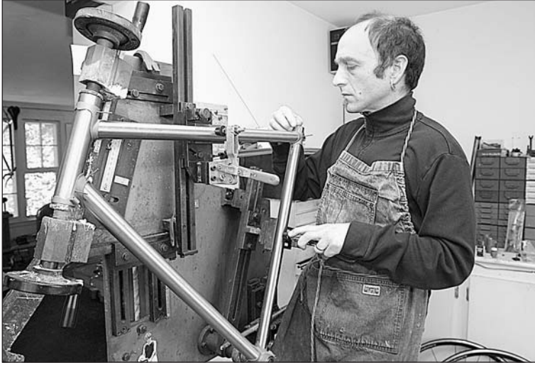
Richard puts pins in the lugs before brazing. "Pinning" the frame helps the set the geometry before brazing. Another way is "tacking" the tubes in a fixture that holds them properly.
