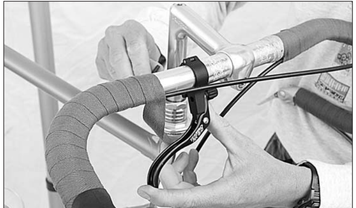
Mount the new lever. Here we're putting it just outside the bar sleeve, but spread them more if you like, or if you're using a Boxy Bag.
