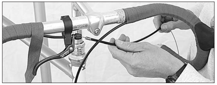
Get another section of housing, prep it and put a cap on it, and run the cable through it. This is the rear one. The other end goes to the housing stop on the top tube. Get the length right.
