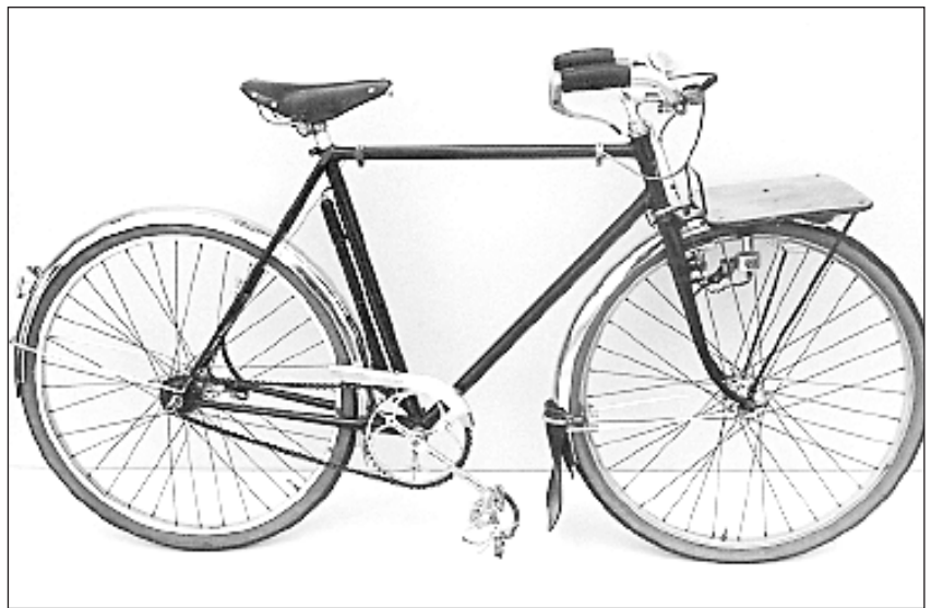
A Goëland Porteur, equipped for the job: Sealed bearings in hubs, bottom bracket and even the pedals meant the owner could deliver newspapers in any weather and not worry about the bike breaking down. Goëland frames were every bit as nice as the top makers', but "budget" parts like steel cranks kept the price significantly lower than that of a Singer or Herse.
