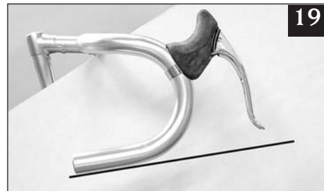
19 Where do the levers go? It's up to you. I like to position it 1-1.5cm above the bottom of the bar, as shown. The "traditional" position is level, but higher supports your hand better. Then, rotate the bars up so the ends point toward the rear brakes. On most bikes, that's about 10 degrees from horizontal. Look at the beautiful curve on this bar.
