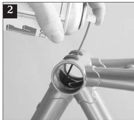
We Boeshield all the frames thoroughly, turning them this way and that to make sure the rustproofing gets into all the corners.
