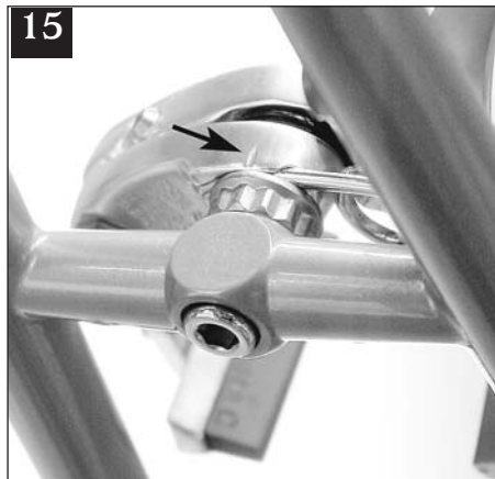
15 The brake is centered when this mark (arrow) is centered. There's a fine adjustment, which we'll get to later. For now, center the caliper and tighten it.
