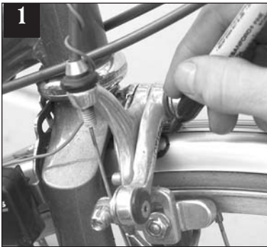
1 Hand-fit the front one under the brake and mark where the brake'll hit.
