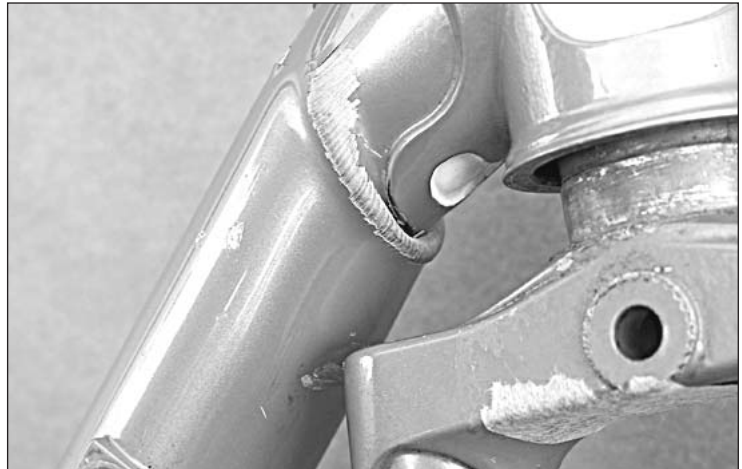
Top: A slight bulge in the rear part of the top tube, just ahead of the lug point. If this were the only damage, the frame could easily be ridden. During riding, the rear of the top tube is the least stressed part of any frame.
