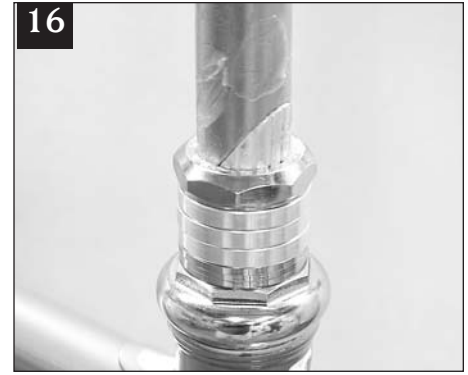
16 Stem into quill: I grease it up good, getting grease on the threads of the expander bolt and all over the wedge, even between the wedge and the quill. Grease, lanolin, or Phil oil work fine. Oil the expander bolt threads if you're fanatical. It cannot hurt.
