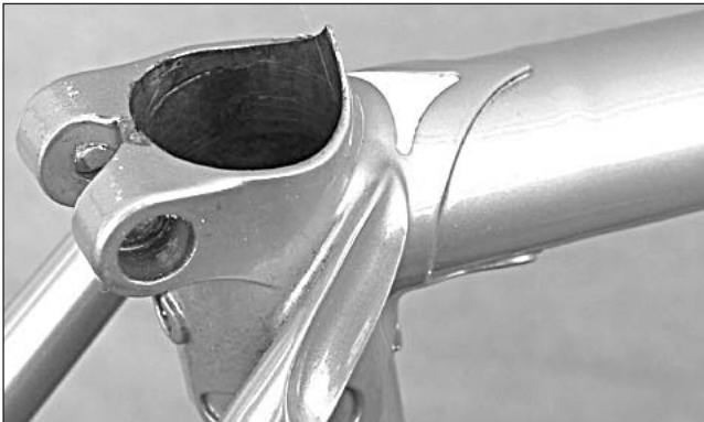
Top: A slight bulge in the rear part of the top tube, just ahead of the lug point. If this were the only damage, the frame could easily be ridden. During riding, the rear of the top tube is the least stressed part of any frame.
