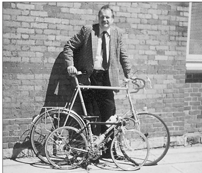
The smallest (34cm) and biggest (87cm) Mariposa bicycles ever made. The customer is David Aird, and he is just under 7 feet. From a builder's point of view, the tough part here is getting a steer tube long enough for the head tube, and finding a seat tube long enough. Most seat tubes stop at 65cm. My guess: Plain-gauge aircraft CrMo reamed at the top to hold a seat post.
