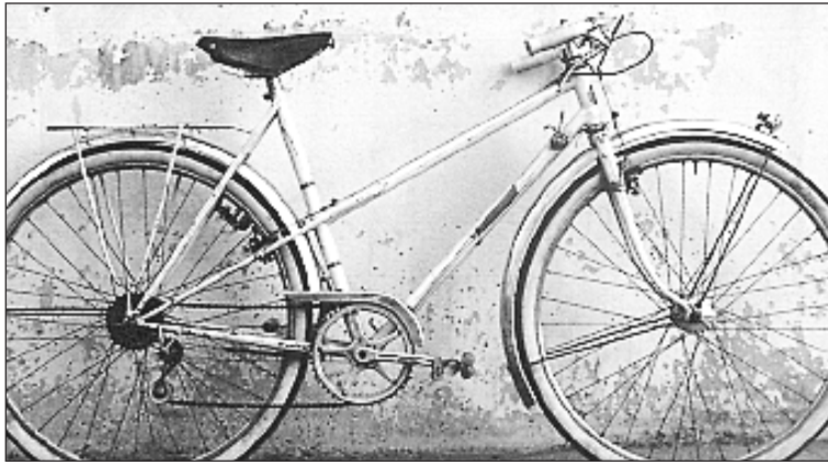
Ondet city bike with a typical performance mixte frame: A diagonal tube meets the seat tube, and additional seat stays brace the rear triangle. This lightweight frame is complemented by top-drawer components: Maxicar hubs, Mavic fenders, cotted alloy cranks, Ideale saddle with alloy rails, cantilever brakes.
