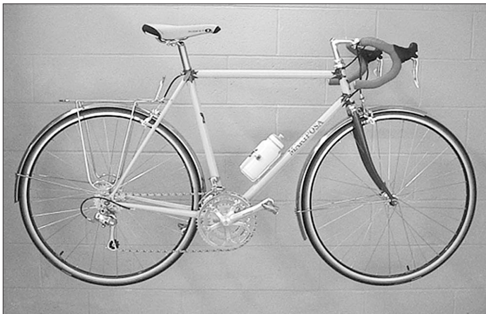
A modern Mariposa road bike, set up for brevets, and built with a mix of components and accessories you don't often see here in the states. Namely, the rack and fenders, with Campy Ergo.
