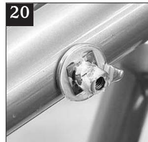
20 Anywhere there's the potential for metal-to-metal contact, I prevent corrosion and frustration by greasing one surface before assembly. I also put beeswax on the screws, both to prevent corrosion and to keep them from loosening. Sometimes the square hole in the washer here is tight on the boss. File it or tap it on, using a socket (or dumbbell) and light mallet.
