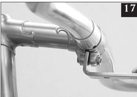
17 The Nitto Stem Pry: Japan's gift to bicycle mechanics, especially those who have ever had to install a Nitto handlebar shim. Even if I'm not installing a shim, this tool is a joy to use. The handlebars go right in, no scratching or swearing.
