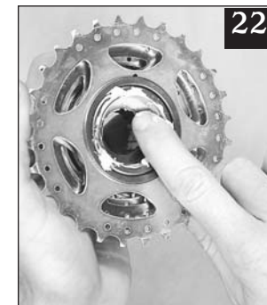
22 Grease the threads when installing a freewheel or cassette! Or use anti-seize. It isn't as big a deal for cassette lockrings, because they aren't tightened by pedaling force, but it's still a good idea. For freewheels, just thread them on by hand and use the test ride to tighten them. Cassette lockrings get torqued to 30ft-lbs.
