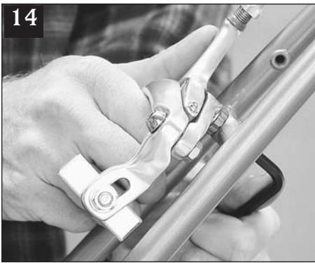
14 Brakes: Just make sure you use the proper washers (or none) to ensure sufficient engagement of the threads. Notice that the pads on these Ultegra standard reach dual-pivots have been swapped out for Mathausers.
