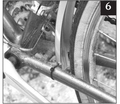
6 Got more zip ties? Use them to attach the rear fender to the chainstays. You'll need to drill holes.
