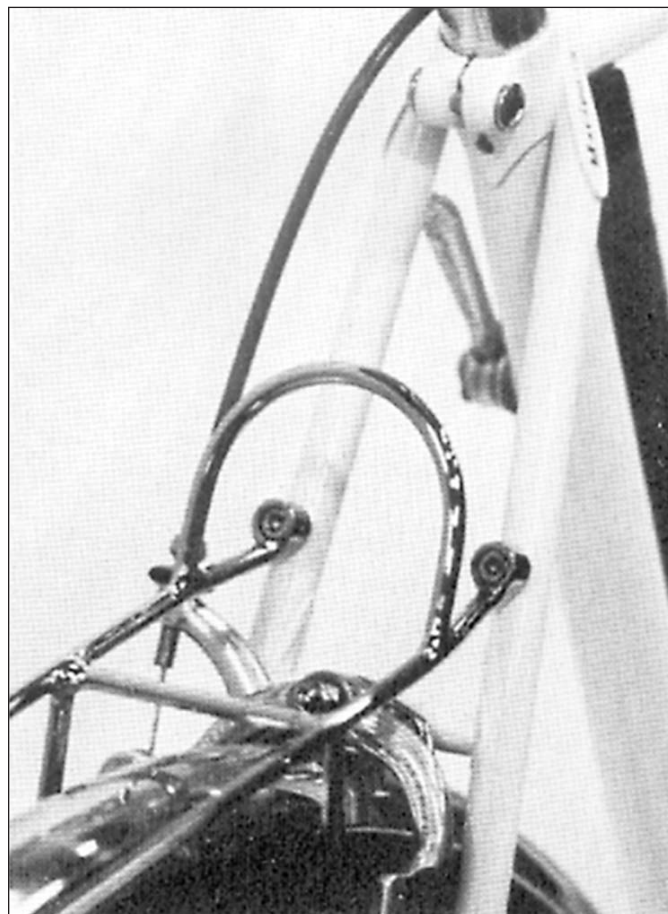
Many Mariposas come with custom racks, such as this one. They're made to fit each frame, and are light and lovely, in the French tradition. I've never seen this particular attachment before. The archy-loop keeps a saddlebag or a rack-mounted load from mashing up against the brake cable or seat stays. Barely in the picture and blurry, you can see the downtube shifter mounted on the upper left of the seat tube. It remotely engages a tire-drive generator, mounted behind the bb.
