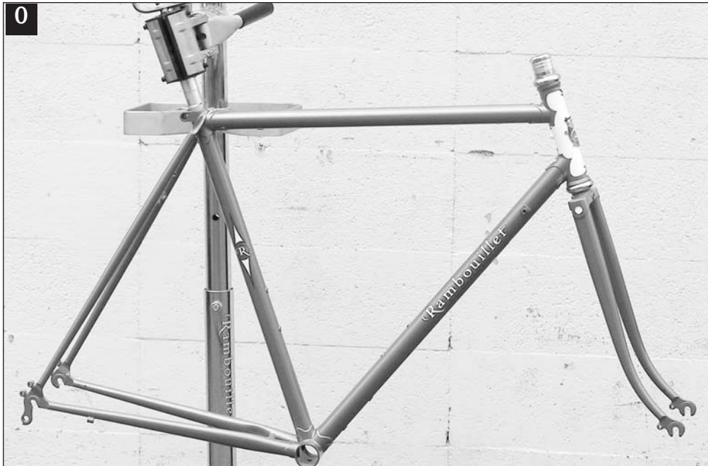
Above: The frame as we receive it. The headset is installed, but may need adjusting and more grease.
