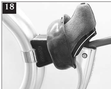
18 Since I only work with new brake levers with fresh and flexy hoods here at Rivendell, I'm comfortable turning them inside out like this for installation. Older gum hoods easily tear, so don't do this with them.
