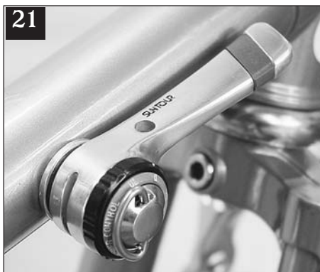
21 Here's the mounted shifter. This one's an old Superbe Pro. On our new Silver shifters, grease the little silver washer, both sides.
