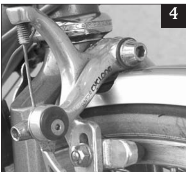
4 With the holes here, the brakes can get squozen without pushing the fender into the tire. This is good!
