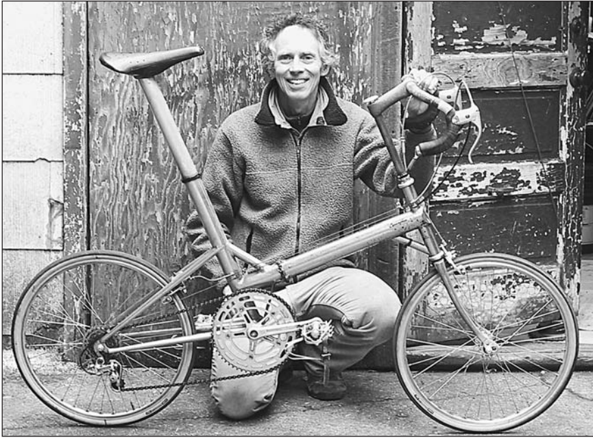
Charlie with the first bike he ever built (1977), and the only steel one. This is a folder with an adjustable front dropout, shown in detail on some other page here.
