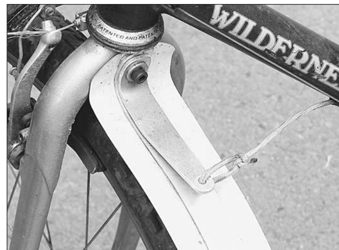
Charlie calls this a "steering limiter." Onto the homemade fender and the back side of the fork, he bolted a tab and tied it to the downtube. It prevents the wheel from turning too much. It's not any sort of a riding aid; just for parking the bike.
