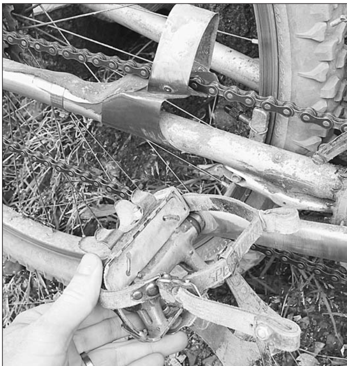
Some early "toe flips" to make flipping up the pedal easier. A makeshift platform for easy in-and-out; a strap modified for grabbing and to keep the hole open wide. Above it, a chain cage to reduce flop and slap. All Charlie made, and typical of the thought he doles out on every part of the bicycle.
