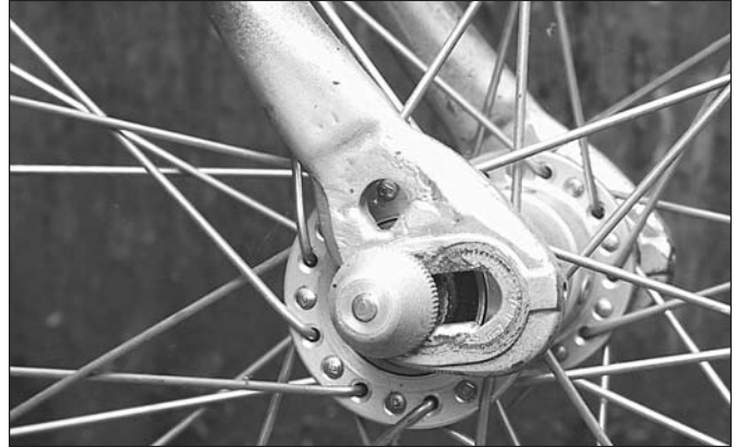
A couple of pages back there's a picture of Charlie with his folder. Here's the front dropout, which allows you to adjust the fork rake. We've been working on one for testing purposes, too...but it may be three or four years until we actually hammer it out. This one's made from a rear dropout. Maybe we should do the same.
