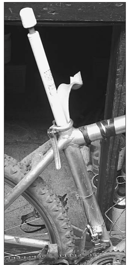
Charlie keeps a full-sized pump inside his seat tube and seat post (not shown). A strip of foam keeps it from jangling.
