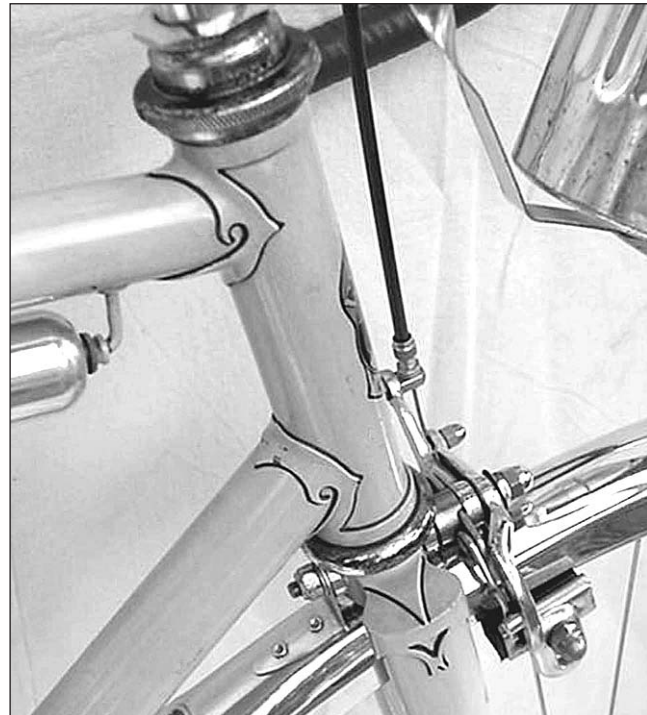
Nice pinstriping and lots of it are the hallmark of many fine English frames. Why get an English bike without it? Notice too, the tiny "bikini" style hand-cut lugs.
