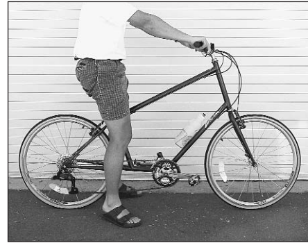
When you can flat-foot the ground like this, the saddle's at the right height for pedaling. This is ideal for children or old people who are afraid to ride normal bikes with the saddle at the proper pedaling height. It's a pretty smart thing, whether or not it's the bike for you.
