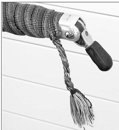
Detail of Bradley's bar wrap, which is a colorful and coarse woven cotton, and his old-style SunTour bar-end Power Ratchet shifter, the original bar-end shifter, and the one Freddie Hoffman (1.3 million lifetime miles and still going) uses on his bike, too.
