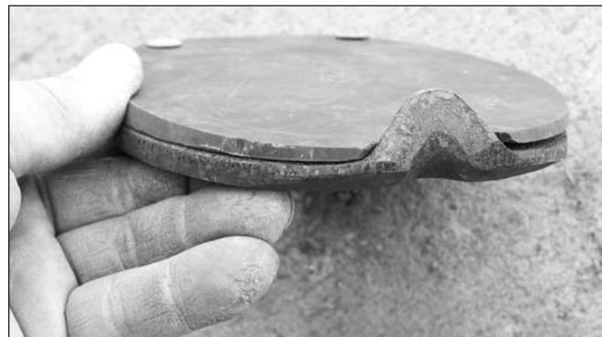
Front view of a shoe made to contain a number of requirements for certification by American Farriers Association. This one has: toe clip, rolled toe (looks like a bevel), wedge pad. Unseen: Welded straight bars and holes tapped for stud calks.
