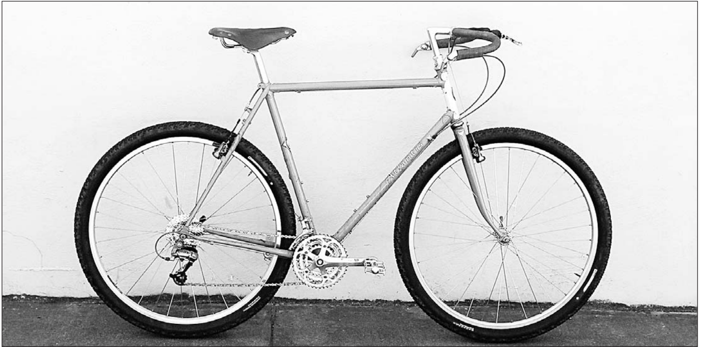
Any Atlantis makes a great mountain bike. The 58s and larger take 700c tires. This 61cm is wearing 700x47/52 WTB Nanoraptor tires & Moustache Handlebars. There are many 700c mountain tires available now, from both WTB and Schwalbe. They're all good, too.
