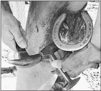
5. Upsetting the nail clinches. In other words, loosening the shoe so you can get more easily get at the nails.
