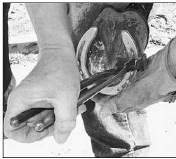
6. Using special pull-off pliers, gently tug the shoe away from the horse's foot.
