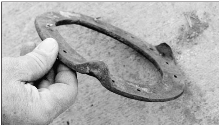
A steel egg-bar I welded up, with hand-forged side clips to help stabilize the shoe.
