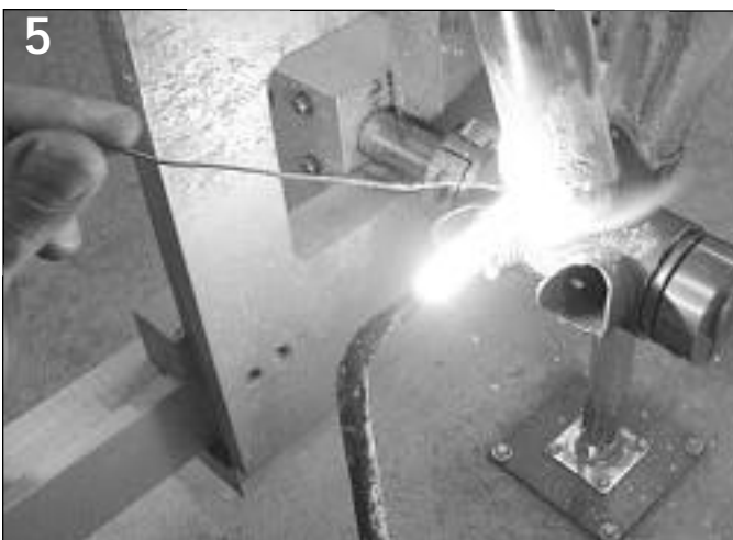
5 Tacking the backside of the seat tube. My right hand is holding the torch and my left hand is holding the silver.
