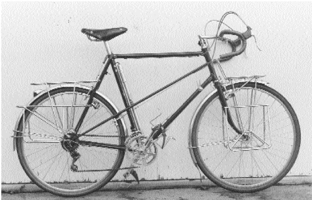
Photo 1: Loaded bike: With 32 quarts of soy milk on board (80 lbs.: 50 in the front panniers, 20 in the rear), this bike handles great. The rear low-rider lowers the center of gravity and greatly improve cornering.
