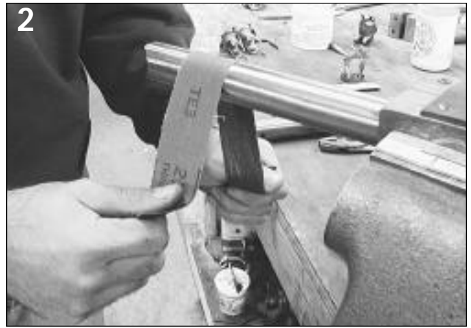
2 Sanding the tube with 80 grit utility cloth. If I had an assistant, this is one task I'd hand off.
