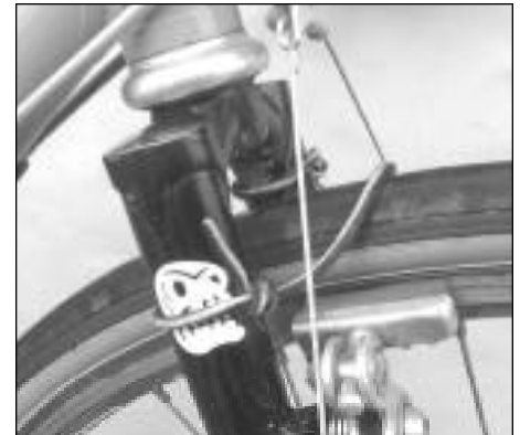
Forkmount. The classic. Slide the knot up and down on the blade until you find nirvana. A 2-3 twist timber hitch is a good knot. Don't know that knot? You should've bought our knot book!
