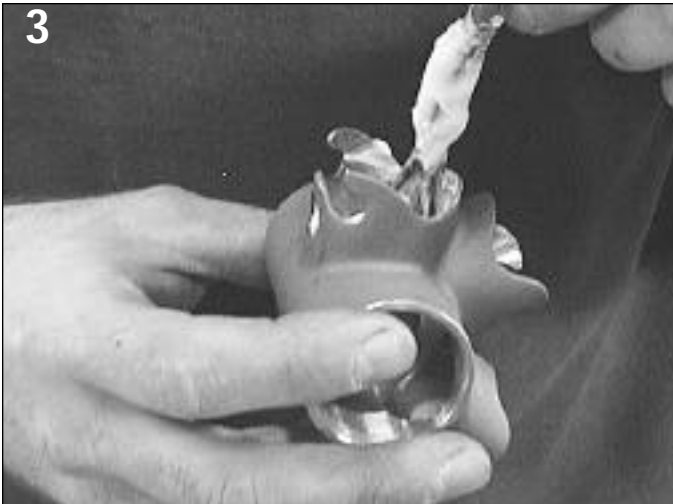
3 Applying silver flux to the BB with a brush. I do this to the tubes, as well. Silver won't flow where there's no flux.
