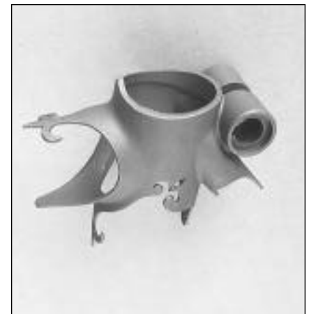
Seat lug. With all the details of the others, plus a binder bolt, and sockets for seat stays. The socket angle is fixed, but the dropouts adjust to accommodate seat stays on small, medium, or big frames.
