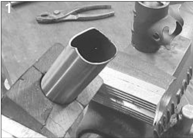
1 This is a seat tube. The second cut allows the seat tube to completely contact the down tube inside the BB.
