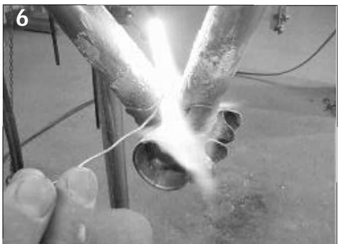
6 Here I'm brazing the BB web. Now the front triangle is out of the jig. I start brazing in the web because this area is 180 degrees from the tacks. Note the clean lug edges!
