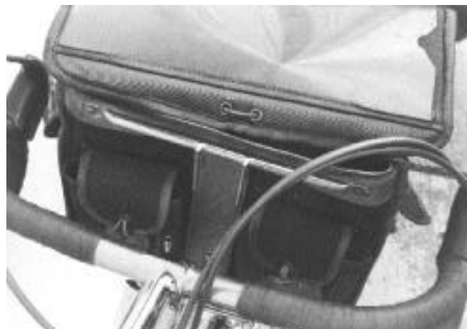
Above: The handlebar bag attaches with an ingenious quick-release. Look careful and you'll see two prongs that fit into the tubes attached to the stem at the bolt. Gravity holds it in place, it never pops off, and to release it for when you want to go into a restaurant for lunch, just lift it up. The Japanese have copied this style for some of their own bar bags. Nitto has made them. Note the permanently attached map case, the fine leather cording around the edges, and the handy elasticated loop closures for the pockets.
