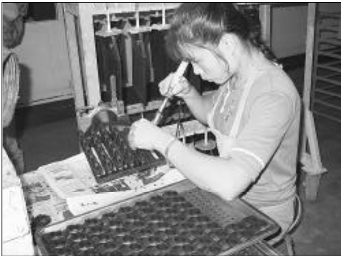
Okay...this woman is using a small heating iron to melt the wax "tree" so she can then attach the wax mold of the lug to it. That way, when they dip it into the ceramic batter, it goes in as one piece. It's delicate work, not easy.
