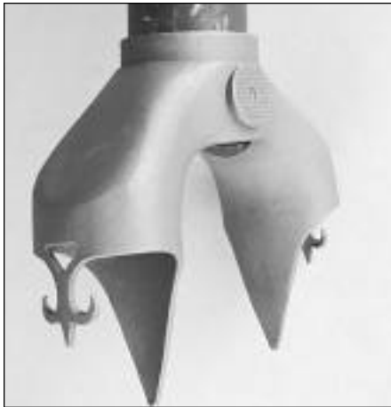
Fork Crown. Full-sloping style for internal fork blades. Oddly, it is cast with an offset, for straight-bladed forks. You'd expect a flat crown designed for raked blades, wooncha?
