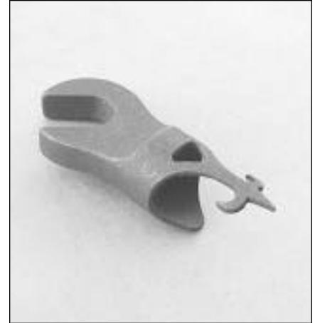
A cast dropout designed to mate with the offset crown. When the blades are straight, you have to angle the slot differently, so it still ends up more or less vertical.
