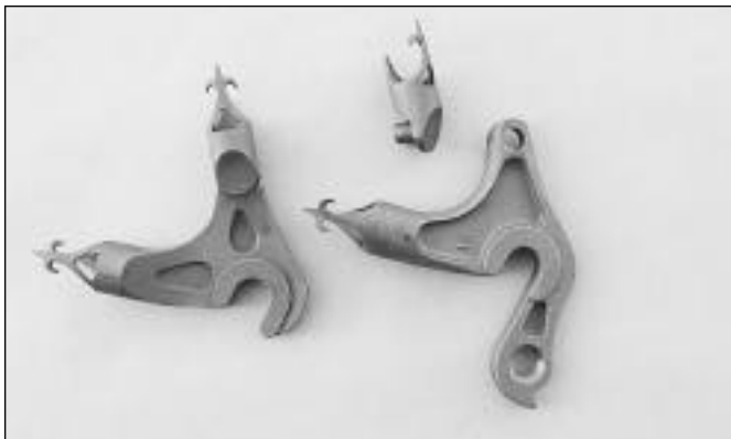
Here dem rear dropouts. The upper socket accepts a seat stay inside it (chopped off straight, no less), and swivels on the main body to accommodate any seat stay angle. Then it all gets brazed. Note also relieved areas to reduce weight.
