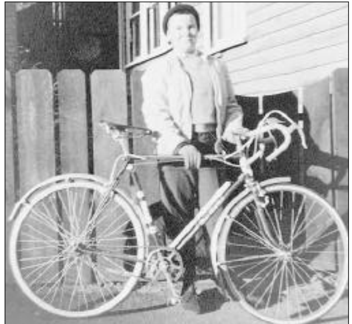
Okay now: The bars are rotated too much and the saddle should be level, but nice fenders, good fork rake, and he's just a kid, for heaven's sake! An Elswick Tour Anglais 4-speed, brand new.
