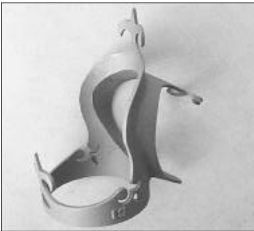
Bottom head lug, showing the anchors, and the crisp bore intersection—a characteristic of cast lugs, which aids brazing. There's no "gap to fill."
