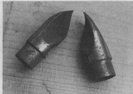
STUBBY ARROWS. The concave areas mate to the seat lug. Lots of contact. See a finished one at this same location on the facing page.
