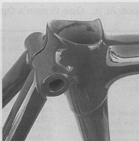
Ritchey Annapurna, Tom's fanciest bike. Note points on the seatstays, a trademark. Combo lug/fillet frame. Tom has always used fastback seat stays. It's his style.
