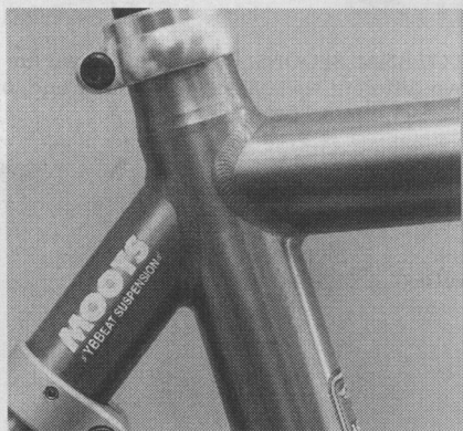
MERLIN/MOOTS. The single tube is welded directly to the seat tube, and in this case, houses a rubber bumper rear suspension
