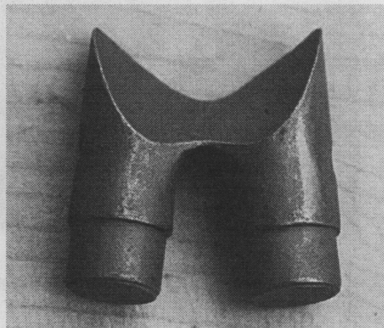
FASTBACK. There are other way to do “fastback” seat stays, but this one’s easy. Braze the upper portion directly to the seat tube, chop the stays off straight, and it looks a lot more labor-intensive than it is.
