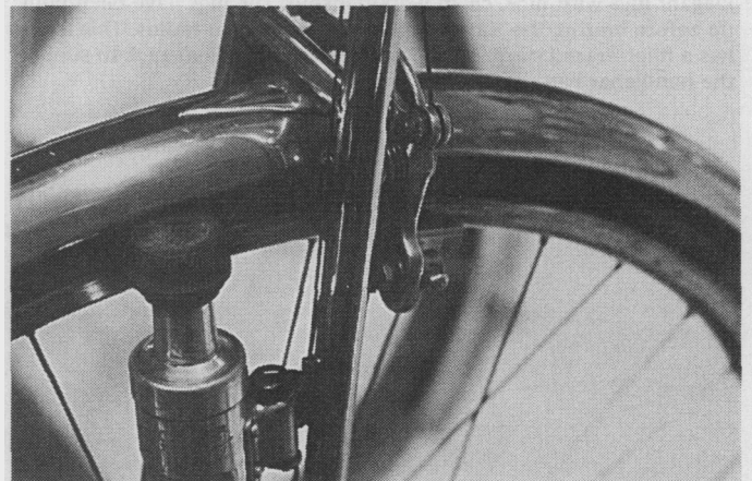
Another 1950s Singer, this one the personal bike of M. Csuka, the builder himself. It's his main bike, and he rides a lot. Note the reinforced fender attachment, remote control for the generator and brazed-on Mafac centerpulls.
