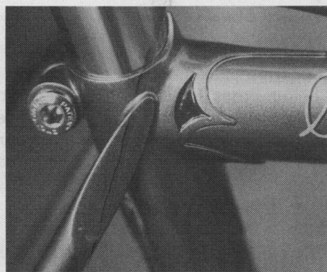
Richard Sachs. The plug is simple and fine. Shown on one of RS's Anniversary frames, built with modified older Riv lugs.
