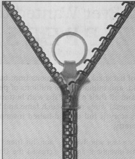
Judson's C-Curly Placket Fastener. Instead of being sewn in by hand, metal hooks were clamped on one side of a cloth tape, metal eyelets on the other. Mated with a slider.
