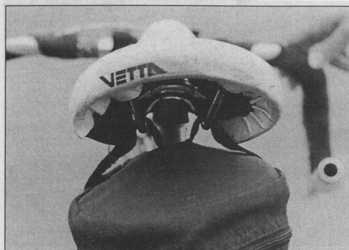
Before: The saddle started shedding its cover—never a good look. Also, notice how round and narrow the back of it is. The new bike needs something better.
