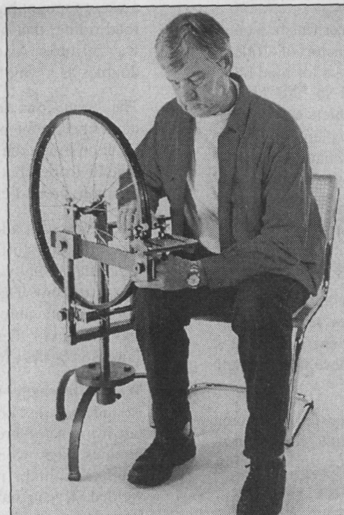
You can turn the nipples and actually watch the rim come into true while you're doing it.
