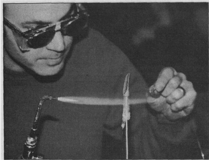
Silver-brazing the plug into the tube. That's a Rivendell-designed plug, only found on Rivendell road frames. The paste on the tube is flux , which may be discussed in another column.
