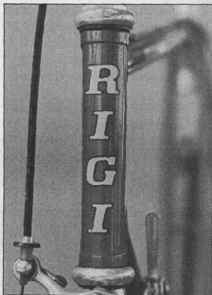
Any kind of lug is better than no lug at all: The Rigi's head lugs are simple, just fine, but a few swirls wouldn't have hurt anything.
