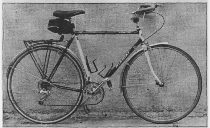
After: We put on a DirtDrop stem and Moustache Handlebars. The steep ramp is gone, the bars are higher, it's better.
