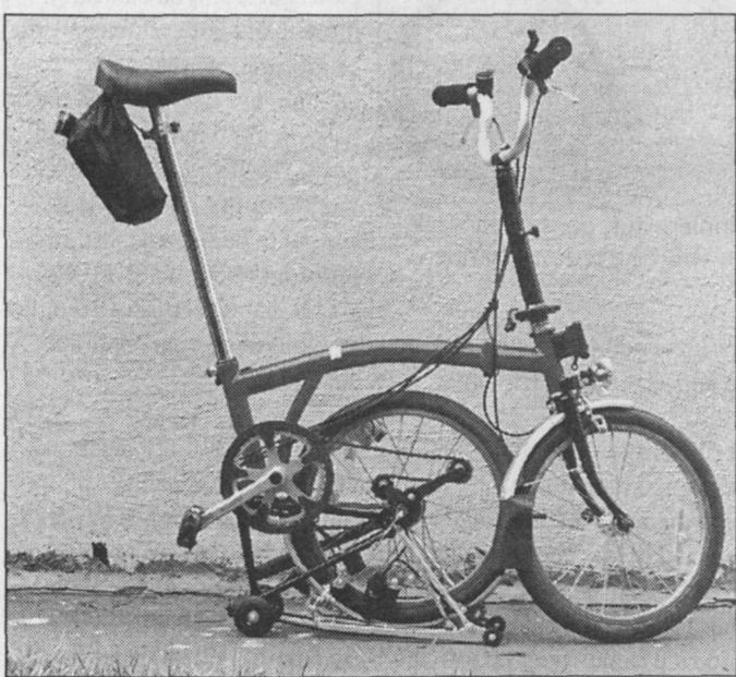
Step 1. Lift the bike and let the rear wheel flop underneath. Turn the front wheel a bit to the left so's the rear don't hit it. The bike rests on roller wheels, and is stable and ready for further folding.
