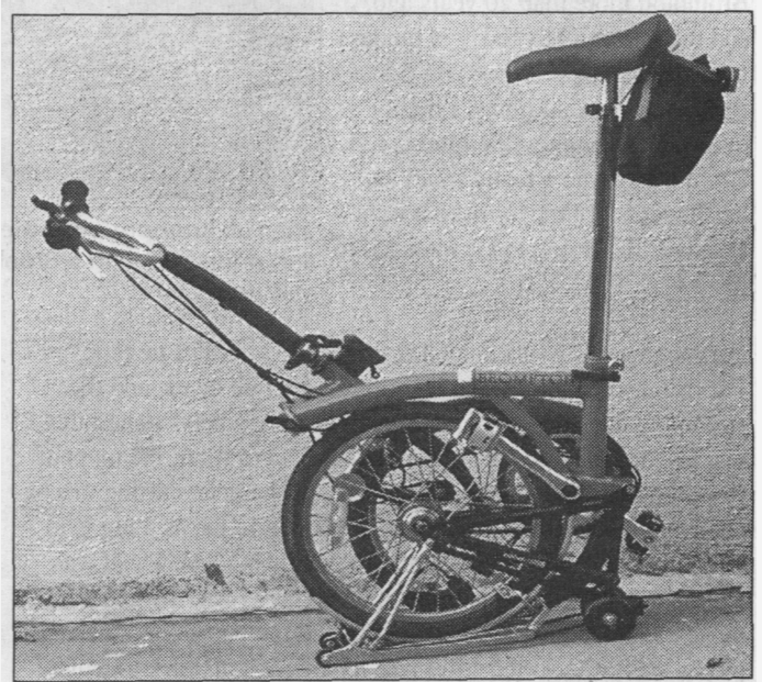
Step 2. Loosen the main frame joint and flop the front half of the bike backwards, hooking a special clip on the wheel axle over a chainstay.
