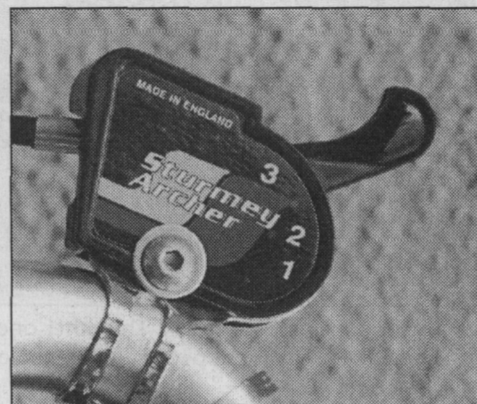
The 3-speed, the classic-and-now-dead-but-there-are-still-many-in-the-pipeline Strymey-Archer trigger shifter. Unchanged for a century or so. Strymey-Archer invented the planetary gear, without which your SUV wouldn't be able to wiggle its way through that preschool parking lot.
