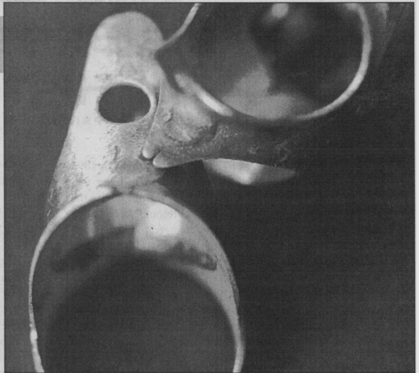
C. Two more lugs that, by modern standards, are substantially substandard. There was one of these on each lug, and builders grew to hate them, since getting rid of the seam took time which could better be spent brazing or mitering—necessary work. Such crummy lugs did not result in crummy frames, though; just as excellent lugs don't by themselves don't make a good frame.
