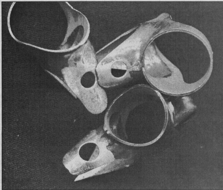
D. These are the rounded spoons on the undersides of each lug. Most Italian lugs have shorter tangs with sharper points; but this is a better design. The three holes were unusual for Italian lugs.
