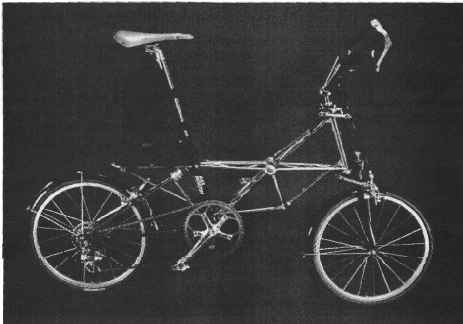
The most recent Moulton, with the airplane-style handlebars and rubber torsion linkage front suspension.
