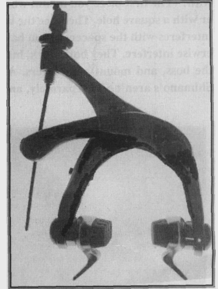
Campagnolo Chorus Mechanically excellent and visually spectacular, but incompatible with fenders. You can barely get clearance when the brakes are open, but as soon as you apply the brakes, the calipers push the front of the fender down onto the tire. Too bad.
