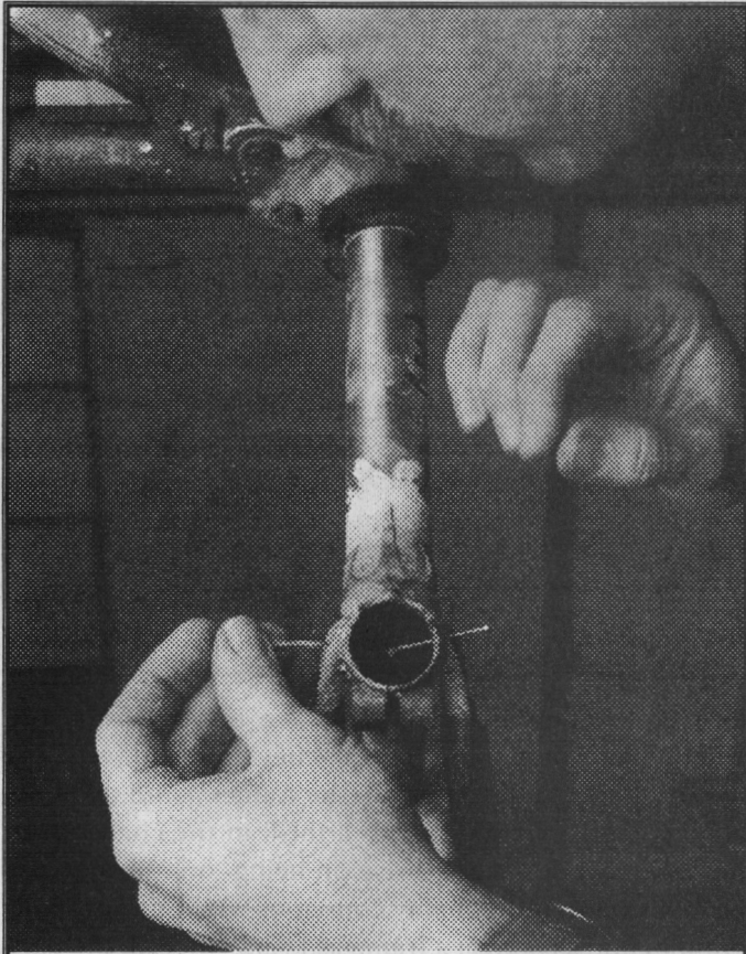
The seat stays are nailed, then brazed, for a solid connection.
