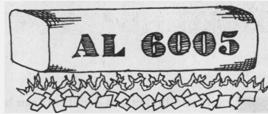
A typical pr-rim billet is 6" x 24". It's heated to 980°F to prepare it for extruding.
