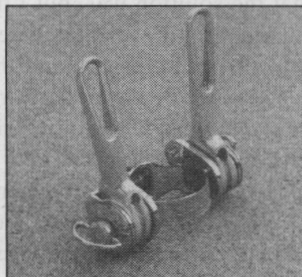
Jubilee shifters. You could remove them from the clamp and put them on braze-ons. You can't do that with others, but it's a typical Jubilee detail.
