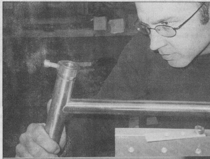
When you TIG-weld, you're pretty much ready to start right now. Here Curt looks at the miter, sees that it's perfect, and the work is about to begin. A lug fits over the joint, and Curt brazes it all together, creating something strong and beautiful. The importance of a perfect miter is debatable, but Curt (and Joe) make them perfect, just in case.
