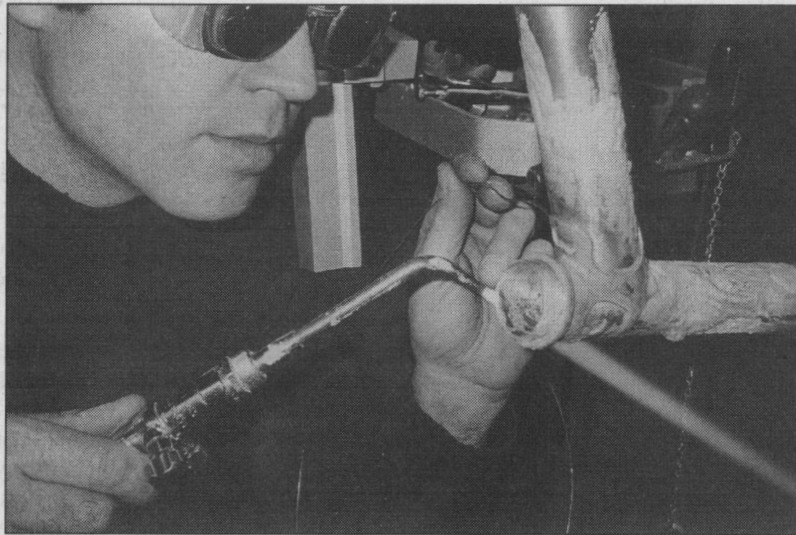
Preparing to braze the lower head lug. The white frothy stuff is flux, which protects the tube from the flame's heat, and creates a favorable environment for brazing.
