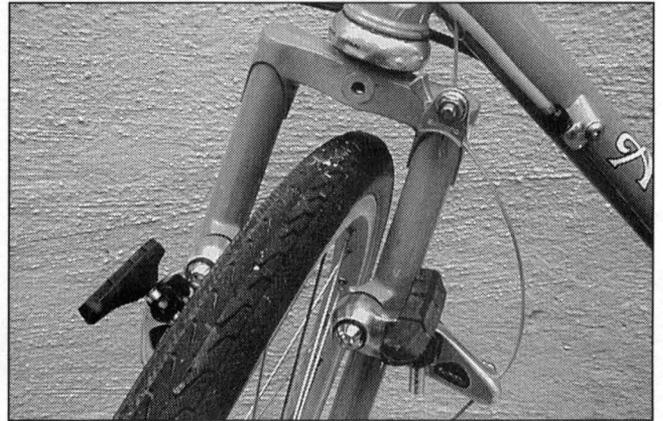
Unhookup the brakes. This is easier with cantilevers or V-brakes than it is with sidepulls, but you can figure out a way with sidepulls, too. Using the barrel adjuster and quick release, loosen them so they don't stop, or snug them so the wheel won't roll.
