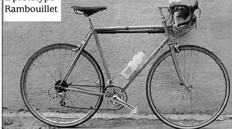
Main tubes have 0.9mm butts and 0.6mm bellies. Seat stays are 16mm x 0.8 single-tapered. Chainstays 0.9mm. Fork 1.2mm. All tubes CrMo. Seat, downtube, chainstays are heat-treated.
