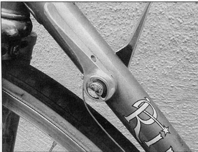
Move the shifters to extreme positions without shifting. Then the fellow will get confused and possibly even consternated when he tries to pedal. Easier with friction shifting. You can tell the left shifter is wacky, because there's so much cable slack.
