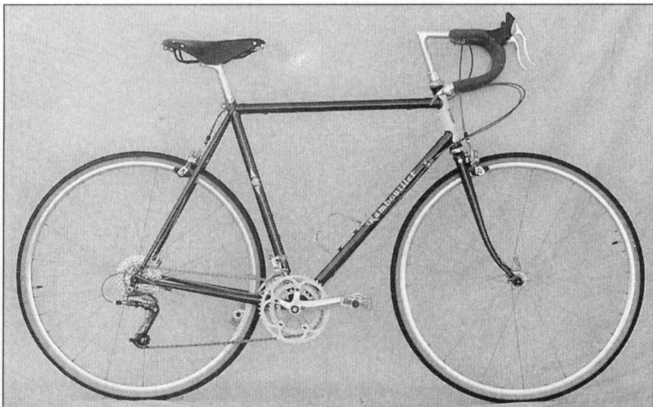
58cm Rambouillet with Ruffy Tuffy tires and low-enough gears for any road riding.
