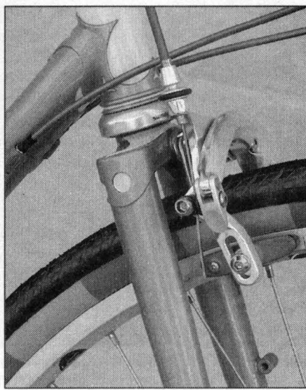
Bottom head lug & fork crown detail.
