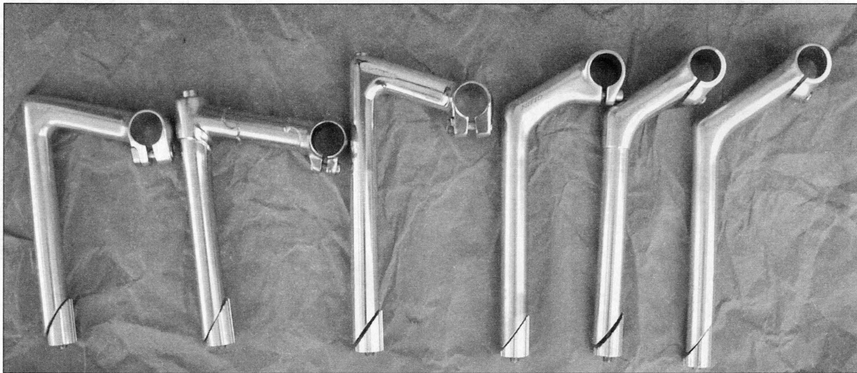
From left to right:: Technomic Deluxe. Lugged, Normal Technomic, Periscopa, DirtDrop 8cm, DirtDrop 10cm. You'll see the bottoms of the stems aren't exactly all at the same height, but the point here is that the DirtDrops and Periscopa really jack the bars up. But even the Technomic Deluxe, shown here as the lowest, gets the bars much higher (almost two whole inches) than a normal stem—a Cinelli, for instance, or a normal clamp-on stem.
