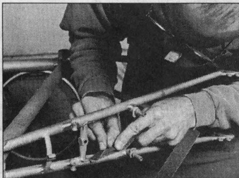
Curt files the edge of a non-essential seat stay bridge reinforcement.
