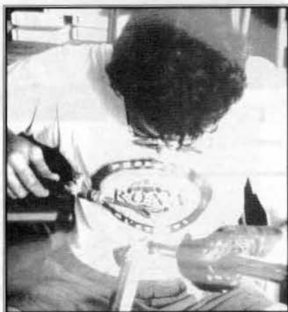
T.R. impersonating Tom Ritchey brazing a head tube joint.
