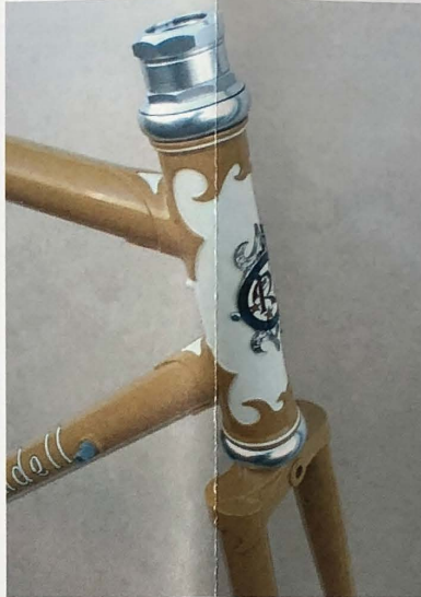
CUSTOM BLUE. Custom-carved lower head lug. Cutting three lugs this way adds $150 to the cost of your frame; but we can do it. Styles vary according to the builder and his mood (always good!)
