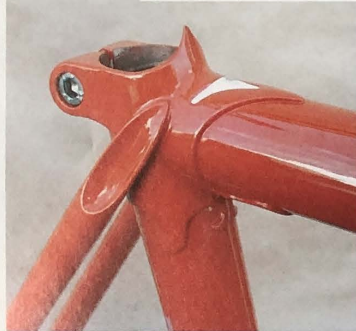
COLEMAN GREEN. Bottom head lug detail, and road crown fancy-cut (see the 3 holes, and the curve), standard paint.(no cream wave on top).
