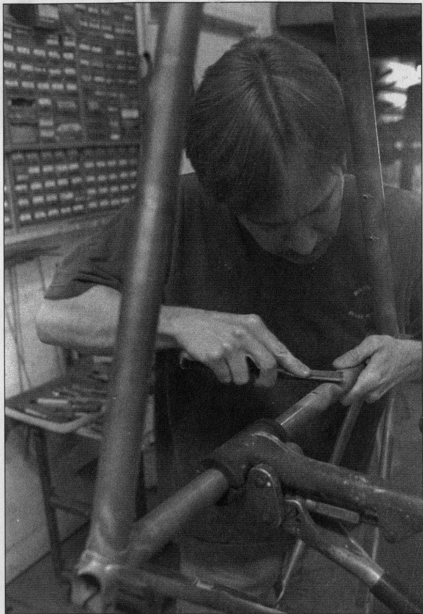
The bottle bosses are reinforced with thin, diamond-shaped plates which must be brazed on separately. Here, Joe cleans up the diamonds, making them extra thin and nice-looking.
