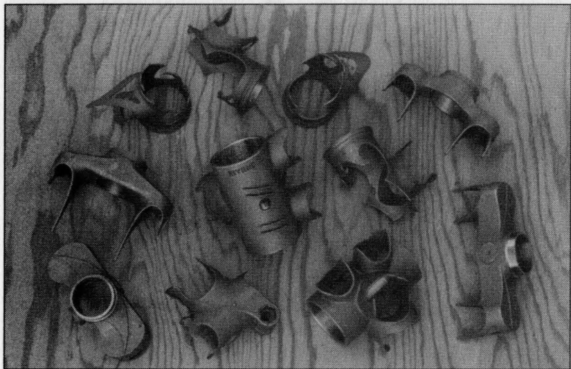
A sampling of mostly proprietary (ours alone) lugs, fork crowns, and bottom bracket shells. The crowns at 2 and 9 o'clock are stock items that made the cut.
