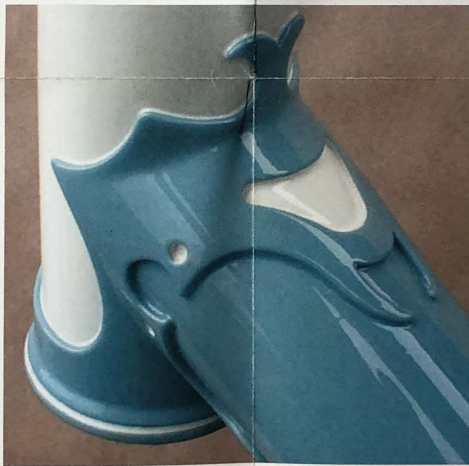
CUSTOM BLUE. Custom-carved lower head lug. Cutting three lugs this way adds $150 to the cost of your frame; but we can do it. Styles vary according to the builder and his mood (always good!)
