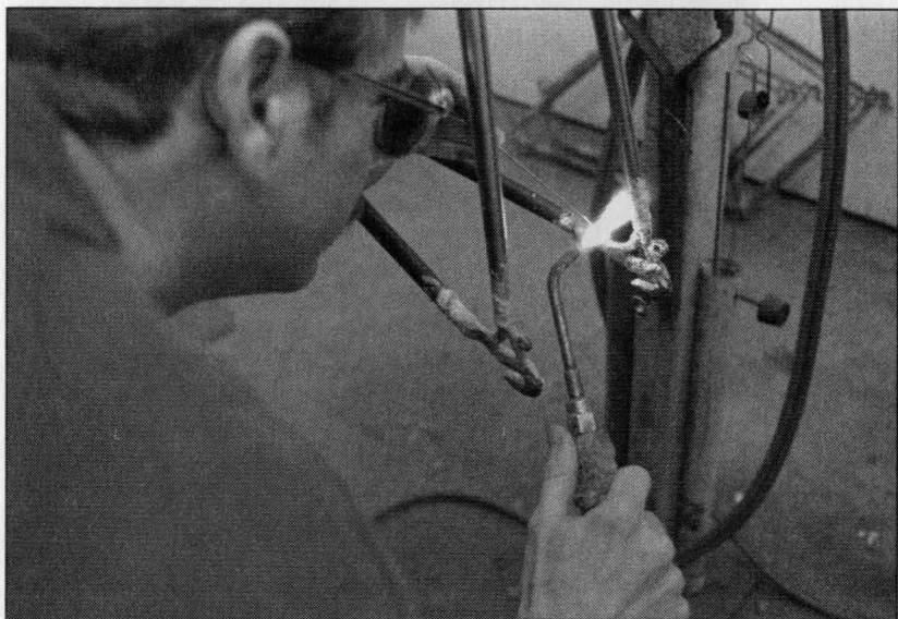
Joe Starck brazing a right rear dropout into the chainstay.
