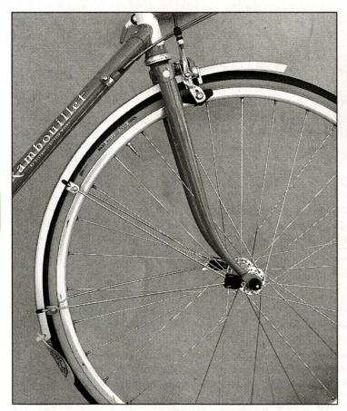
It is easy to mount fenders on a Rambouillet. The fork is the right length, the seat stay bridge (not shown in this photo) is in the right place, and the dropouts have eyelets.
