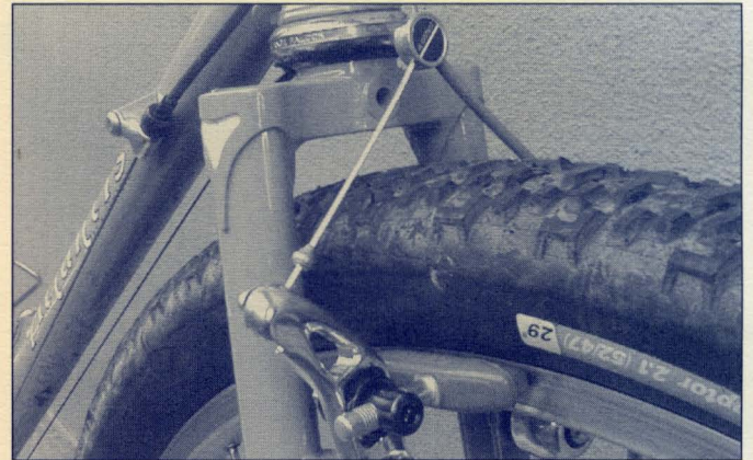
Top: 61cm Atlantis fork with a 700x52 WT B Nanoraptor. Bottom: 56cm Atlantis chainstays with a 26x2.1 knobby. Room for fenders, mud, wobbly wheels. Atlantis frames have great clearance.
