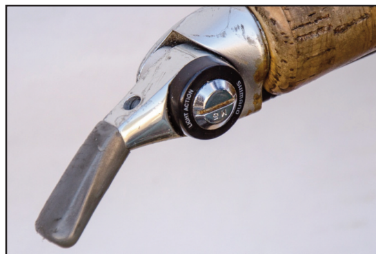
Shimano's bar-end shifter in 8- and 9- speed have index and friction modes. The friction mode is not as luscious as SILVER's, but it works great.
