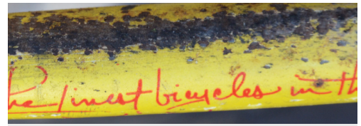
Roman's chain-rattled chainstay on a Nashbar mountain bike. A good case for using a chainstay protector, easily made with handlebar tape.
