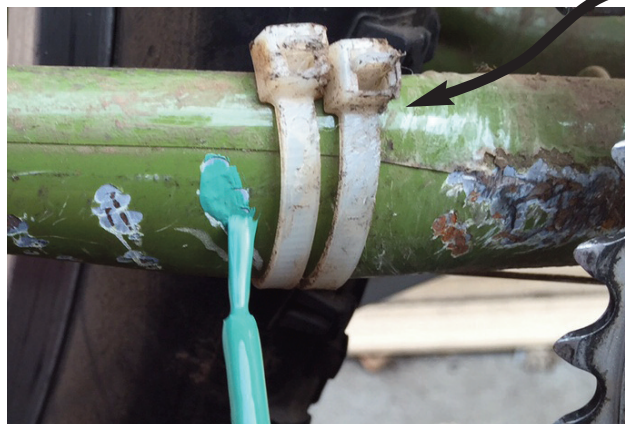
Will touches up the ravaged chainstay on his Hunqapillar. He's using touch-up for an Atlantis, and it'll be fine! Please do us all a favor and ignore the zip ties. They're anti-chainsuck things that either he put on after the fact, or just didn't work. They have nothing to do with touching up the paint.
