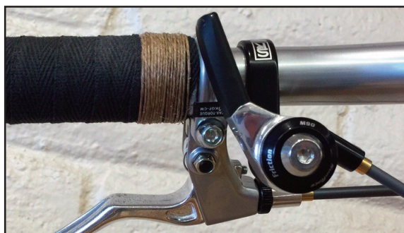
SunRace's friction-thumbies, made at our request (based on an existing SunRace model). Mount the left on the right & vice versa . . . inside the bar.
