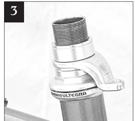
3 Install whatever spacers, then the hanger, and another spacer on top of it, as you like.
