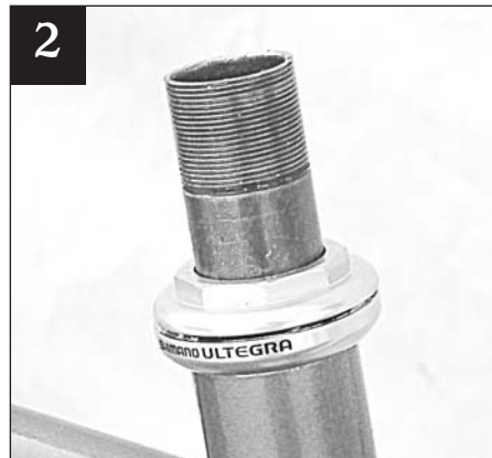
2 Then slide on the now-threadless upper cup. There's no going back now...
