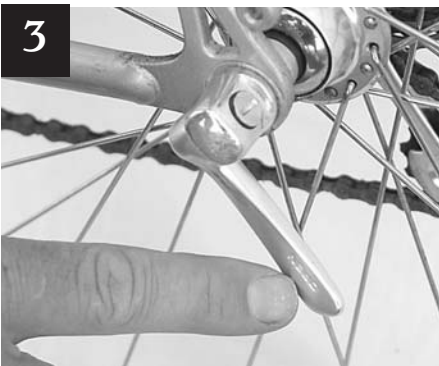
3 Open the rear wheel's quick-release.
