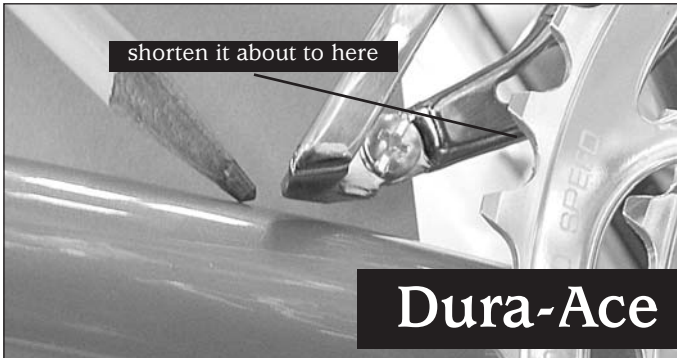
See how close it comes to the chainstay? And that's with the derailleur set too high! Set it right and the tail of the Dura-Ace will hit the chainstay. Shimano could solve this by lopping off 8mm of tail, which would mean you couldn't ride a 26 front x 12 rear combo, but who cares about THAT gear? Compare the tail of this cage with the 105/Ultegra and you'll see the extra length that causes the trouble. Remember now, it's a problem only with sub-50t chainrings on 700c bikes with low bottom brackets. But that rules out some smart bikes and smart gearing. Dear Shimano: Please fix it.
