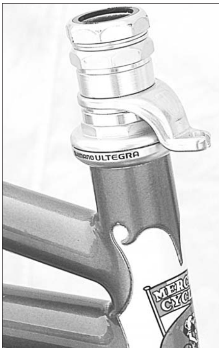
2 Then slide on the now-threadless upper cup. There's no going back now...
