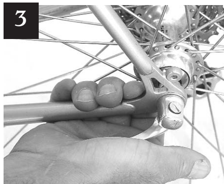
3 Close the wheel's quick-release.
