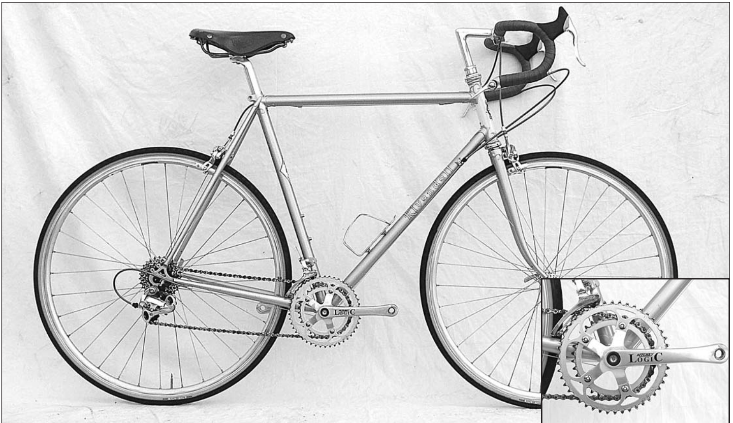
Here's Moe set up as a smart, versatile road double. Ritchey Logic crank, 46 x 34 rings. More specs below.
