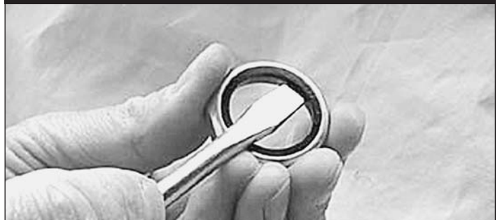
Go to your local bike shop and ask kindly if you might purchase a used locknut from an old headset. If it's not too old, it might have a cheap plastic fake seal in it, and if that's the case, pry it out. If it's a real old model, it may have a lip on it, which you'll need to grind off. This piece will substitute for a Genuine Aheadset's "star-fangled nut," to lock in the adjustment. You must be able to thread it onto a steerer without the plastic seal or metal lip stopping it.
