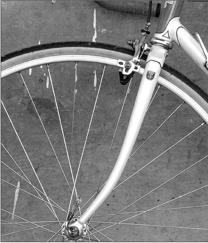
Brand X late '80s. Fatter lower legs, less rake, straight section before the dropout.
