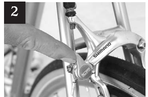
2 Open the brake's quick-release.
