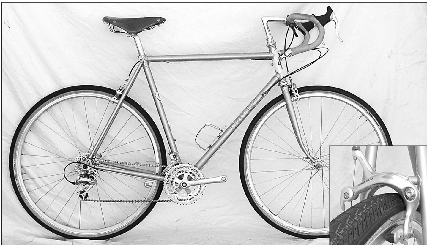
Here's Larry. He's set up for fire trails and bad roads, with Panaracer Pasela 700x37 tires and interruptor brake levers, which you can barely see if you look at the top of the handlebars. More specs in the chart on the next page.
