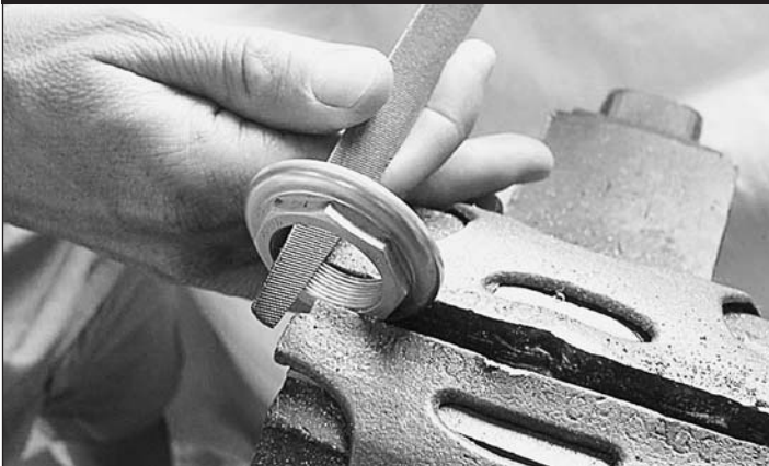
File out the threads from a threaded headset's upper cup. Do not ask your machinist friend to do this for you. You don't even need a vise.
