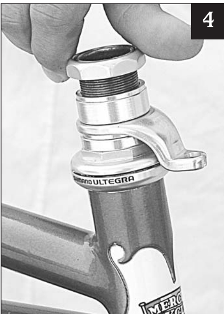
4 Now screw on the spare headset locknut that's been stripped of its seal. This is now a substitute for a "star-fangled nut."
