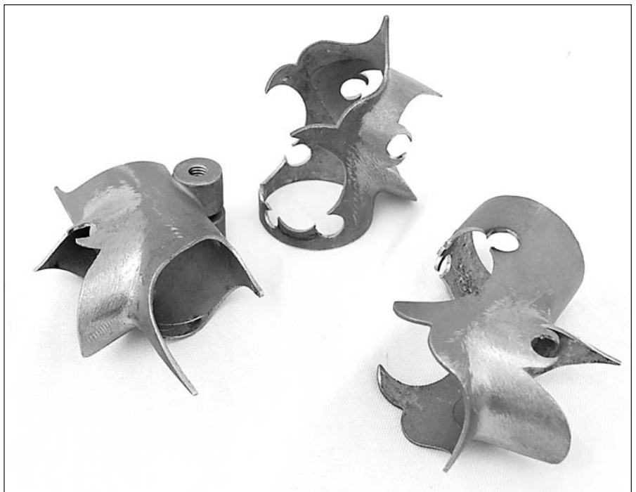
As you know from reading RR29, Richard now has his own new lugs. But these here are his modernized version of the classic Nervex Pro lug set. You can tell they aren't the originals, because they're neat and clean, and have a head tube extension.
