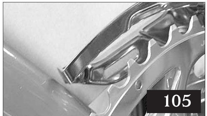
This 105 derailleur's tail comes as close to the chainstay as does the Dura-Ace—but when shifted to the outer ring, the cage is much closer to the chainring, for better shifting. The Dura-Ace is marginally prettier and whoppingly more expensive, but the 105, for our loot, is a better design. The Ultegra, by the way, fits just like the 105.
