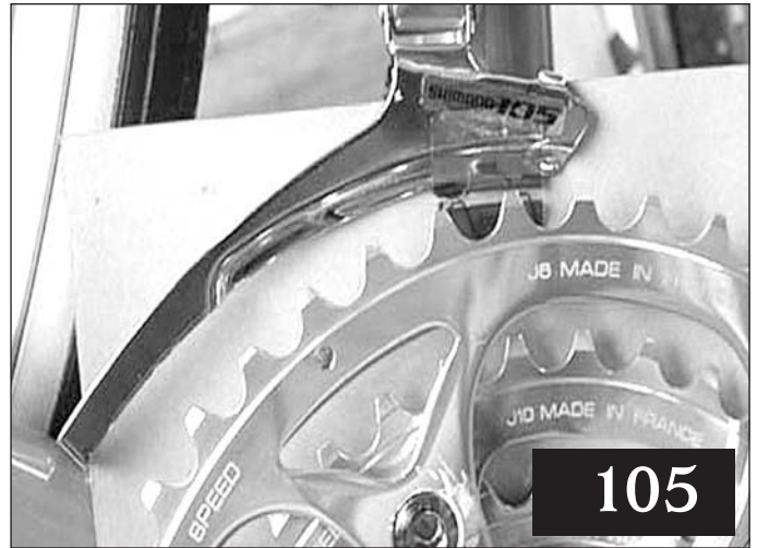
Here's a 105 triple front. It's still higher than we'd like it to be, but it's a lot closer to the ring than is a Dura-Ace. It can be closer to the ring because it has a shorter tail.
