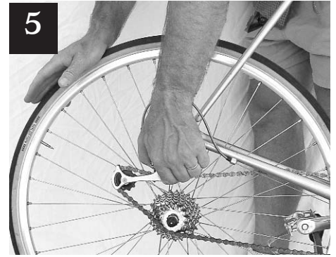
5 Push the wheel down and forward.
