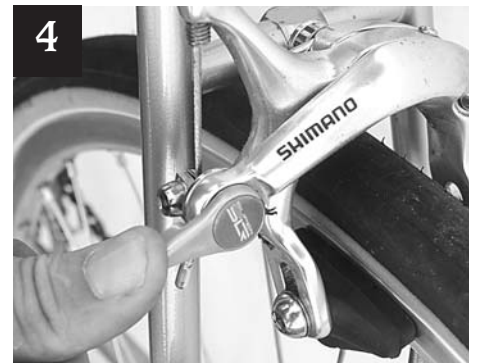
4 Close the brake's quick-release.
