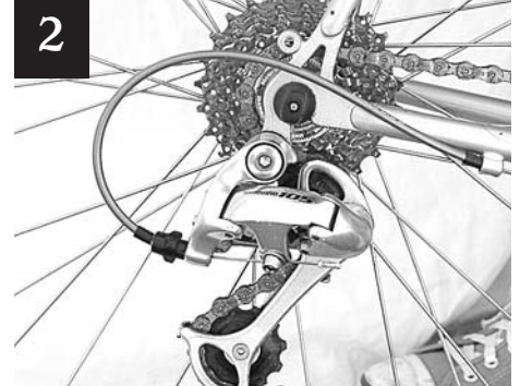
2 Slip the axle into the dropout.
