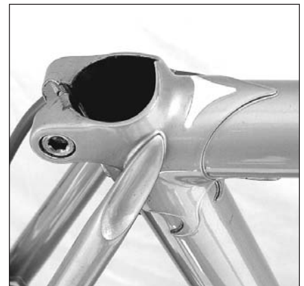
Left: The seat stay brazed onto the seat lug, on a bike I recently finished for J. O. Right: A finished & painted seat cluster made with a plug. Right: A complete and painted Rivendell road seat cluster made the normal way, with a plug. Looks nice!
