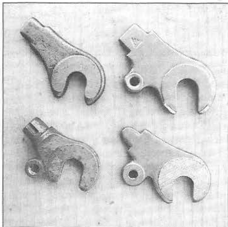
Three tab dropouts, showing tab widths from 13 to 17.3mm. You can't "point" the dropout with the skinny ones. And a plug-style...
