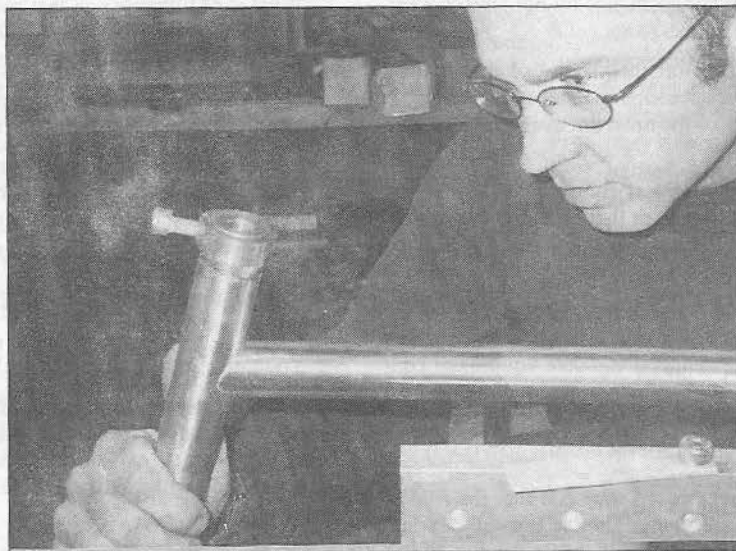
When you TIG-weld, you're pretty much ready to start right now. Here Curt looks at the miter, sees that it's perfect, and the work is about to begin. A lug fits over the joint, and Curt brazes it all together, creating something strong and beautiful. The importance of a perfect miter is debatable, but Curt (and Joe) make them perfect, just in case.
