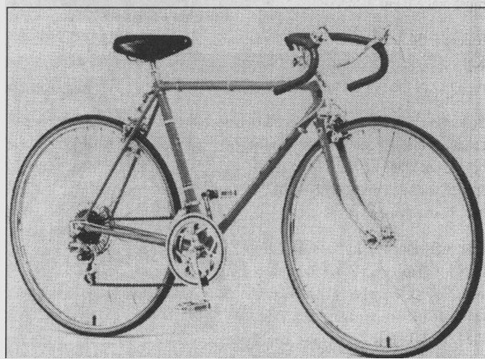
Figure 8. The 1974 Fuji Tourer was a typical low-priced Japanese ten-speed. It had SunTour derailleurs, a Sugino cotted steel crankset with 50-40 chainwheels, a SunTour 14-34 freewheel, a Sunshine alloy quick release, high-flange hubs, and Dia Compe center-pull brakes. The Fuji still weighed more than the Peugeot but the heavier frame could take more abuse. Even though the gear spread was much wider, every writer commented on the smooth shifting SunTour derailleurs.
