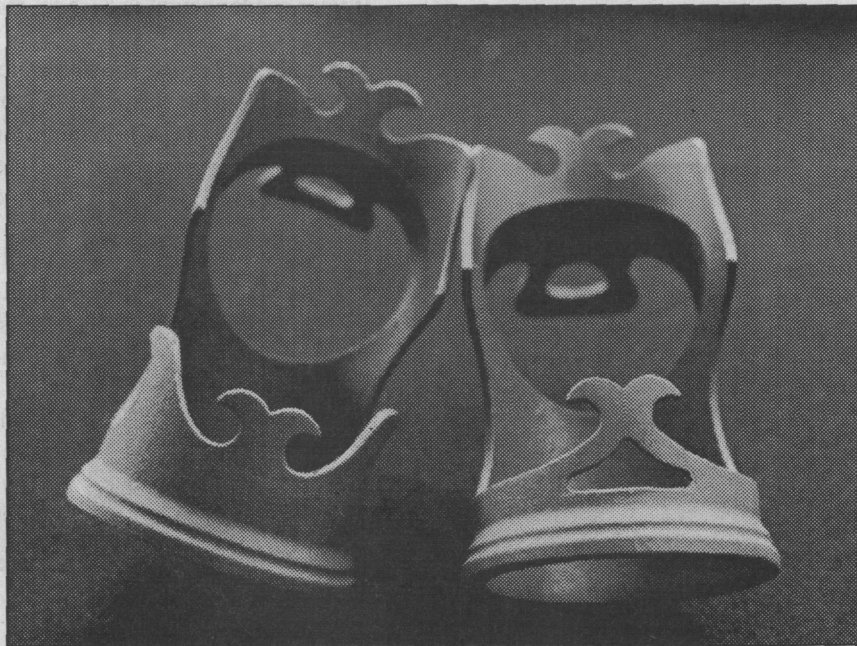
The Atlantis's lower head lug (R) and the Papilio (L). A keen eye will see a similarity. The one on the right is easier to braze, theoretically. The first one will be brazed on January 25th.
