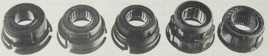
PHOTO 6-5 Wide-spaced freewheel bodies: left to right, Maillard 700 Course (5- or 6-speed); Regina Oro BX (5- or 6-speed); Regina America (6-speed); Shimano MF-Z (6-speed); and Maillard Helicomatic (5-speed).
