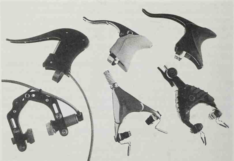
PHOTO 13-1 Unconventional brakesets: left to right, Mathausen Hydraulic, Campagnolo C-Record, and Weinmann Delta Pro.
