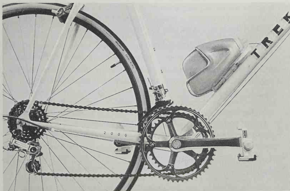
PHOTO 3-3 Alpine gearing on Berto's Trek 2000 racing bicycle.
