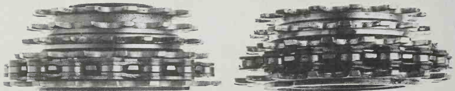
PHOTO 4-2 Chain clearance: left, narrow Sedisport chain in a narrow-spaced freewheel; right, wide Uniglide chain in a wide-spaced freewheel.
